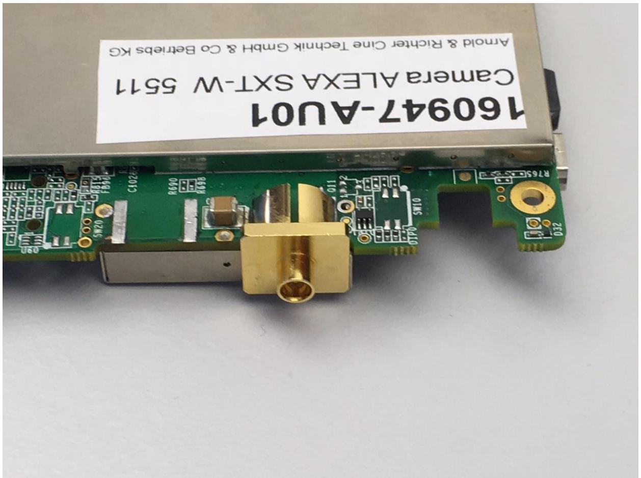
Picture 7: AMN35253_PB_ARRI_B: EUT MCX7 connector
