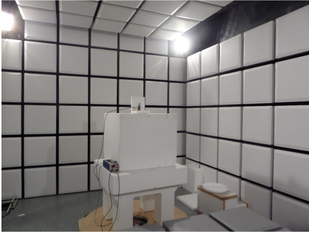
Radiated by structure test: Position 1
