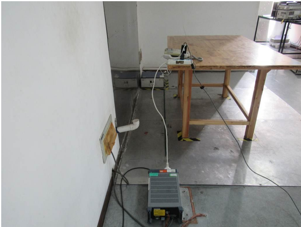
Conducted Emissions Test Setup Side View (Adapter)
