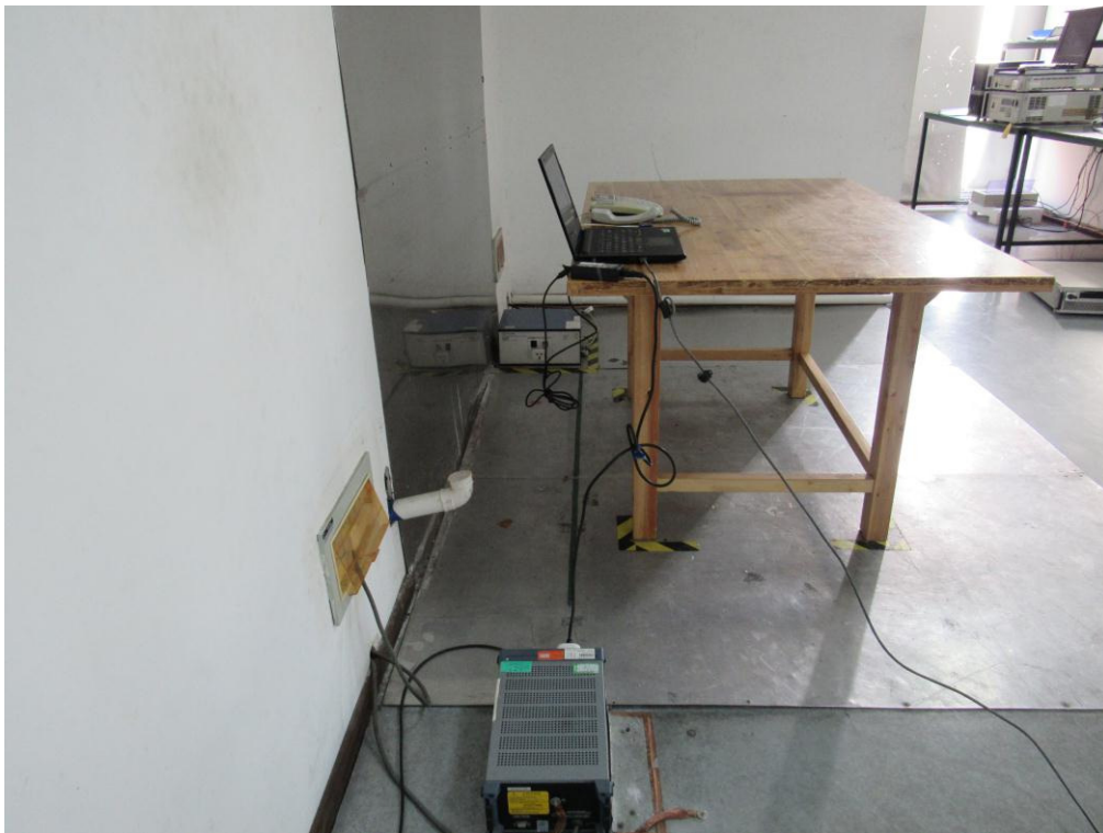
Conducted Emissions Test Setup Side View (Notebook)
