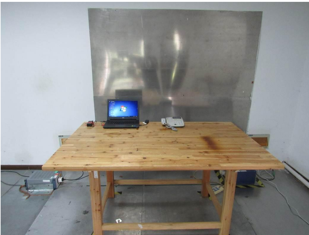
Conducted Emissions Setup Front View(Notebook)
