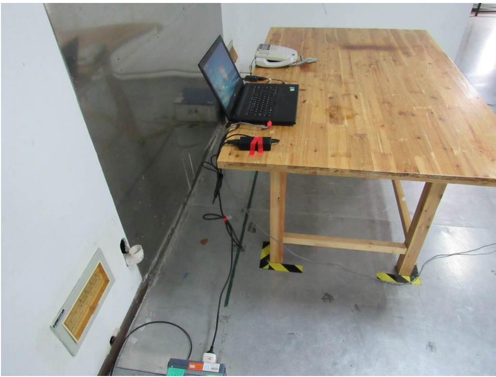
Conducted Emissions Setup Side View(Notebook)
