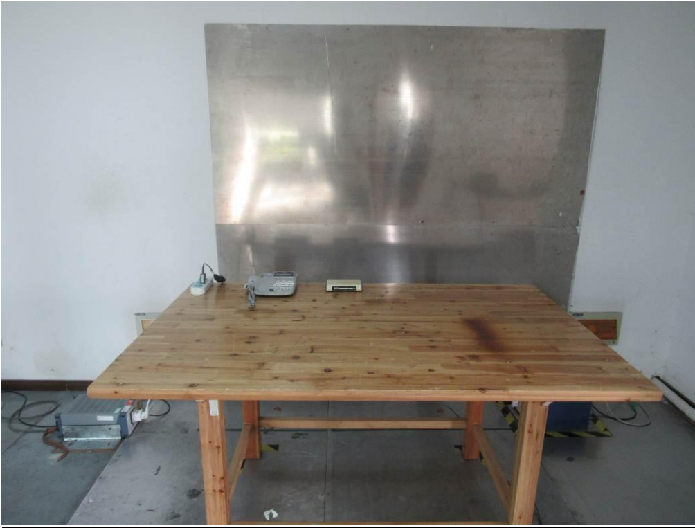
Conducted Emissions Setup Front View(Adapter)
