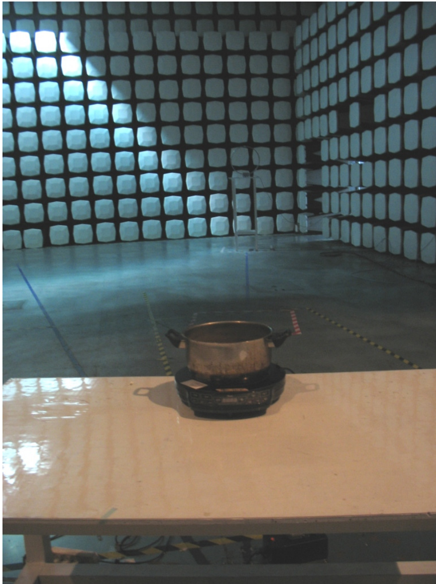
Photograph 2: Set-up for Radiated Emission
