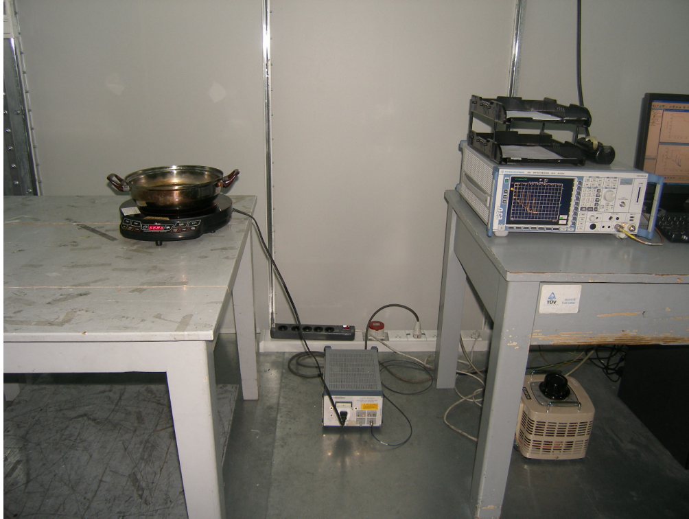
Photograph 1: Set-up for Conducted Emission
