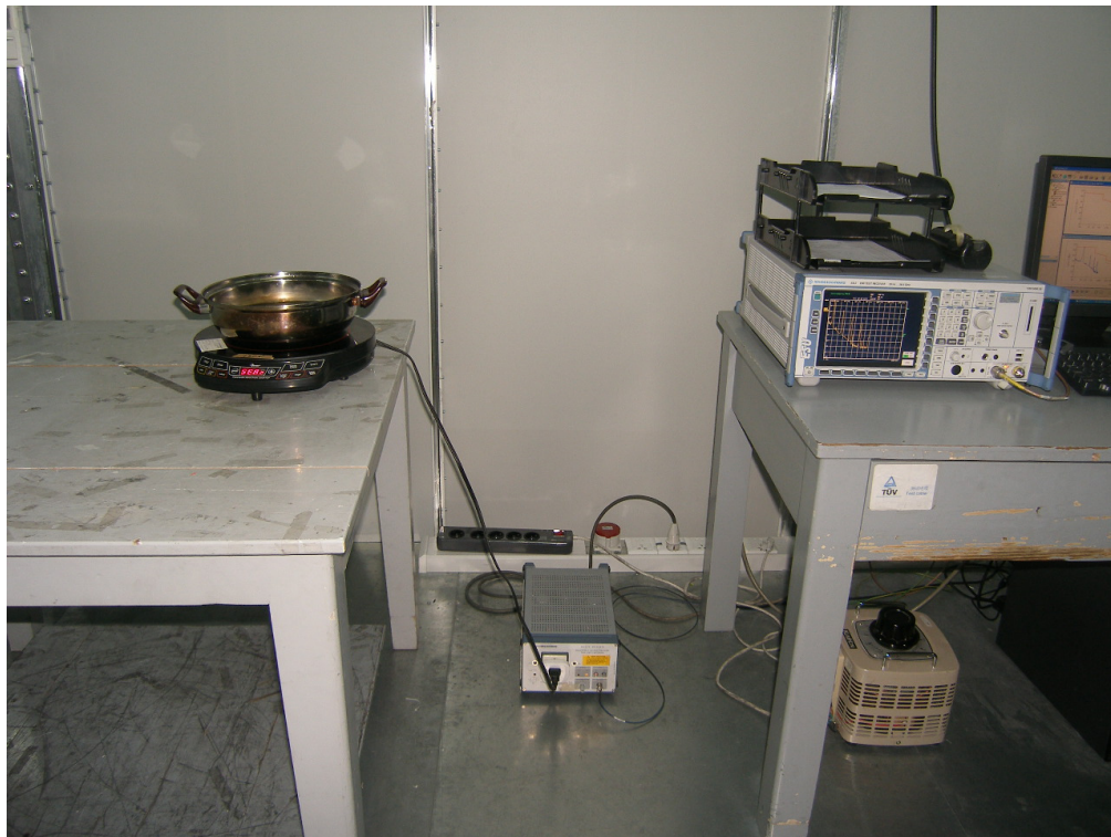
Photograph 1: Set-up for Conducted Emission
