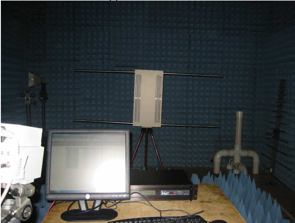
11.32(d): 10 V/m RF field at 1MHz
