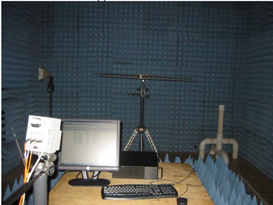
11.32(d): 0.5V/m RF field at 108MHz
