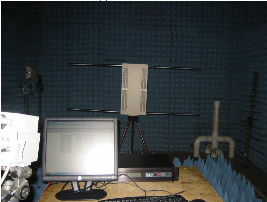
11.32(d): 10 V/m RF field at 1MHz
