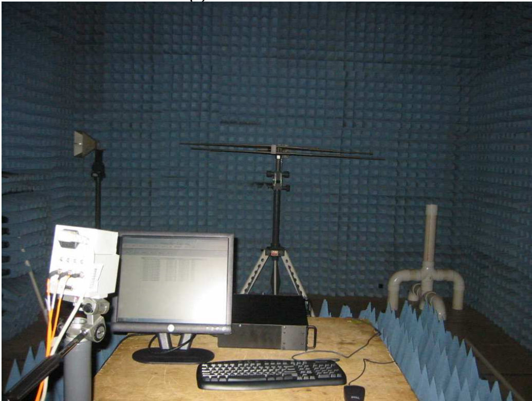
11.32(d): 0.5V/m RF field at 108MHz
