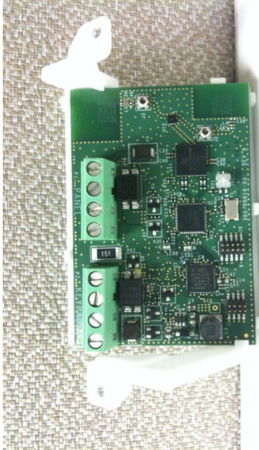
260-00016-04 Zigbee Panel Interface Module in plastic holder 2 nd view
