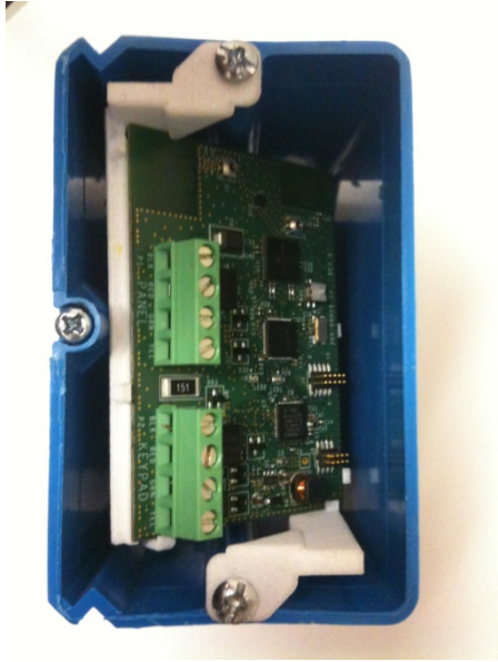
260-00016-04 Zigbee Panel Interface Module in holder mounted in box
