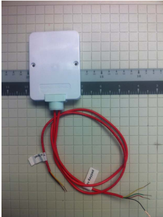
4000001604 v2 Zigbee Panel Interface Module in Plastic Housing Front
