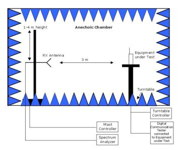
$\underline{\textit{Remark:}} \ \textit{Depending on the frequency range suitable} \\ \textit{antenna types, attenuators or preamplifiers are used.}$
