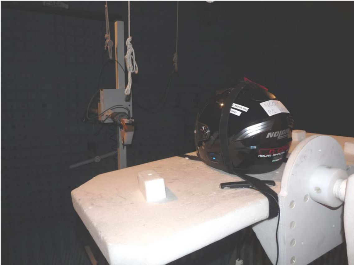
Photo 4: Test setup for radiated measurements (Enclosure, above 18 GHz)
