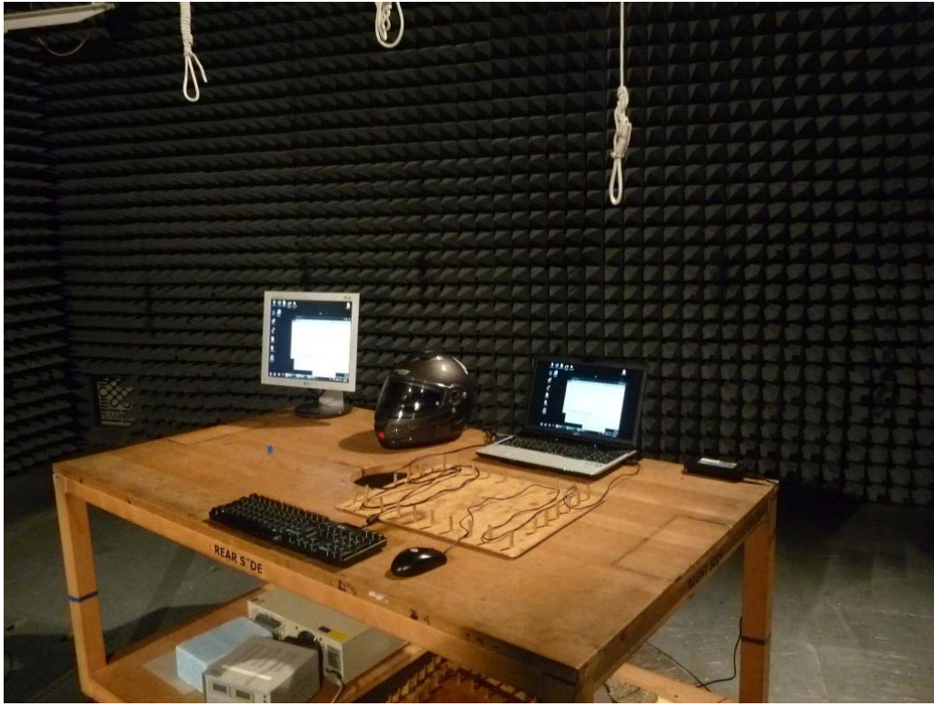
Photo 7: Test setup for radiated measurements (Enclosure, 30 MHz to 1 GHz), unintentional transmission, EUT + computer peripheral setup
