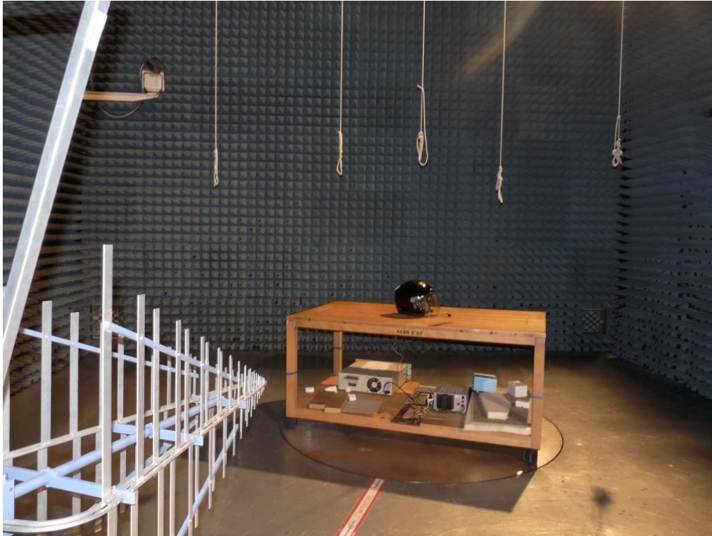
Photo 2: Test setup for radiated measurements (Enclosure, 30 MHz to 1 GHz), intentional transmission
