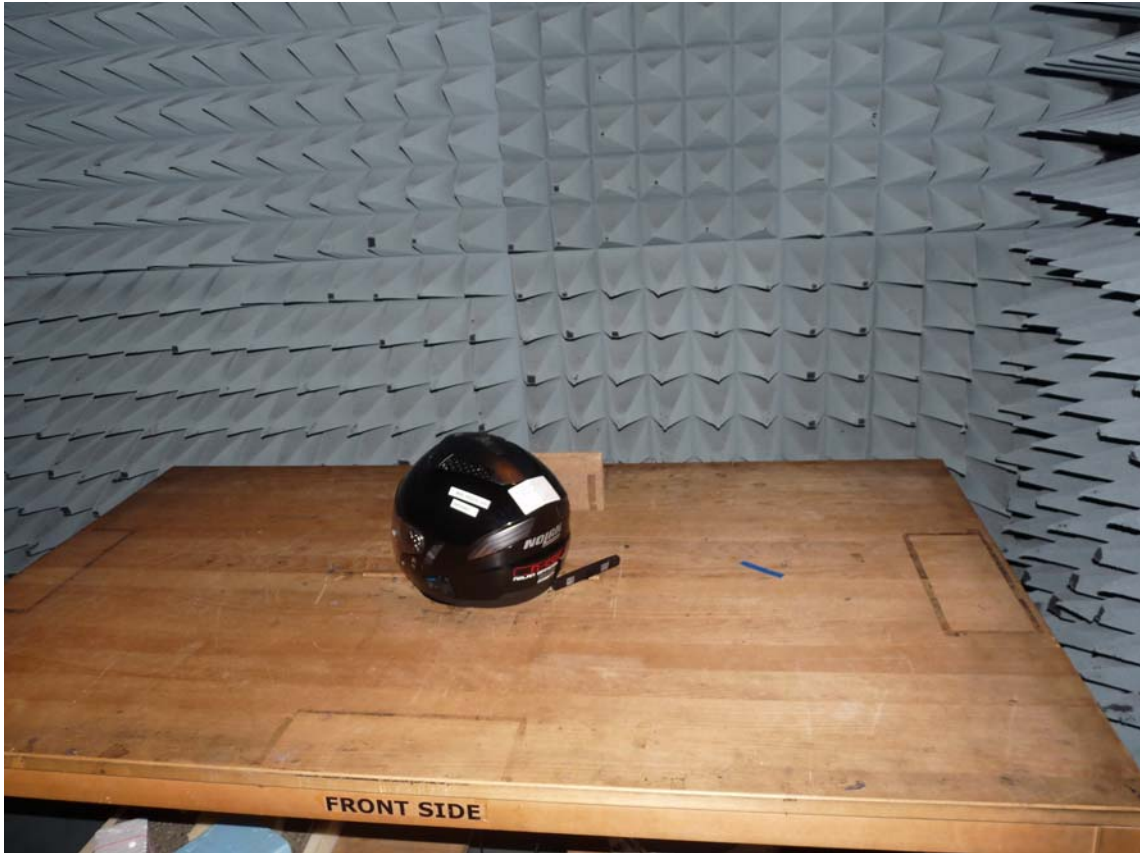
Photo 1: Test setup for radiated measurements (Enclosure, below 30 MHz) Part 15c
