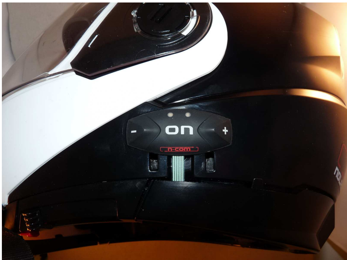
N-COM B4 inside helmet (control buttons on left side of helmet)
