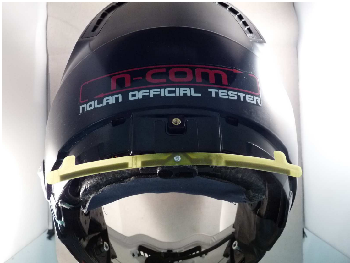
N-COM B4 inside helmet (back cover opened, antenna visible)
