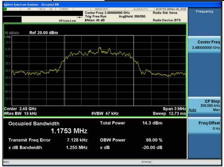
20 dB Bandwidth & Occupied BW <u>Lowest Channel & Modulation : 8DPSK</u>
