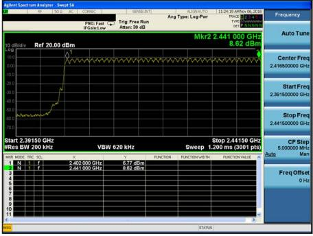
Number of Hopping Frequencies 2(FH) Hopping mode : Enable & π/4DQPSK
