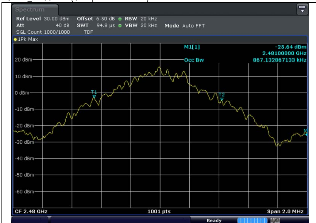
GFSK_2 480 MHz(Occupied Bandwidth)
