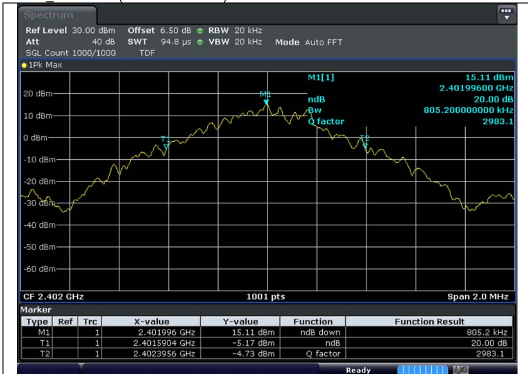
GFSK 2 402 MHz(20 dB Bandwidth)
