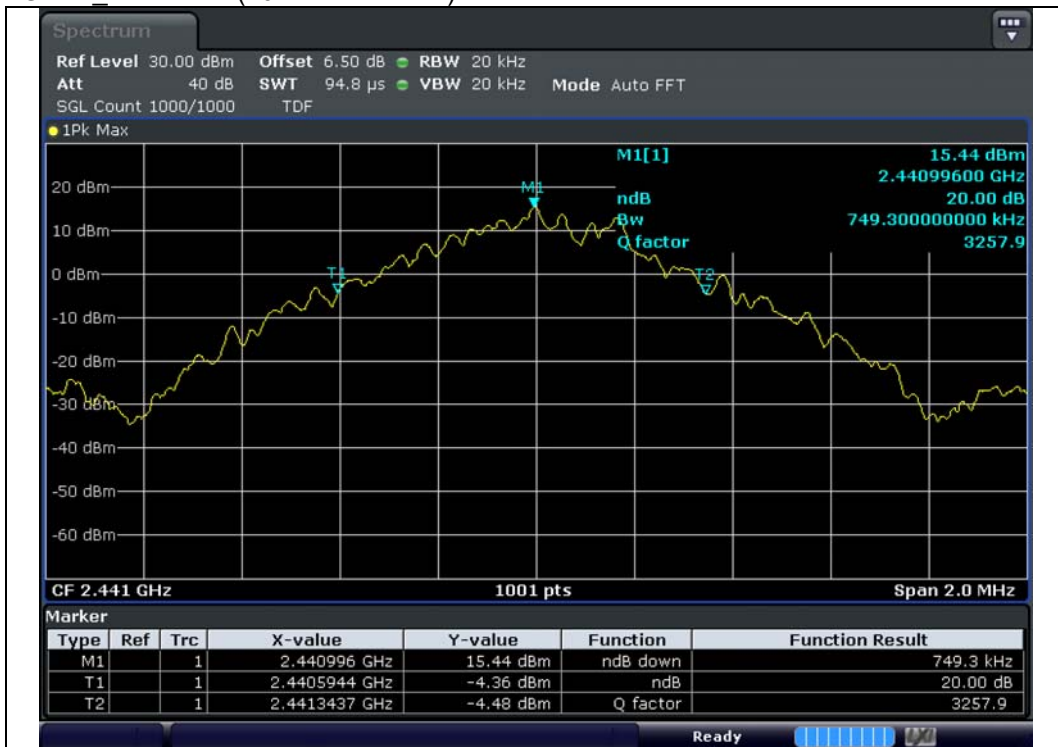
GFSK 2 441 MHz(20 dB Bandwidth)
