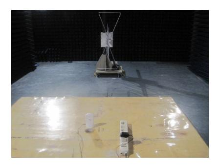
**Radiation Emission Test View For 1GHz-25GHz**
