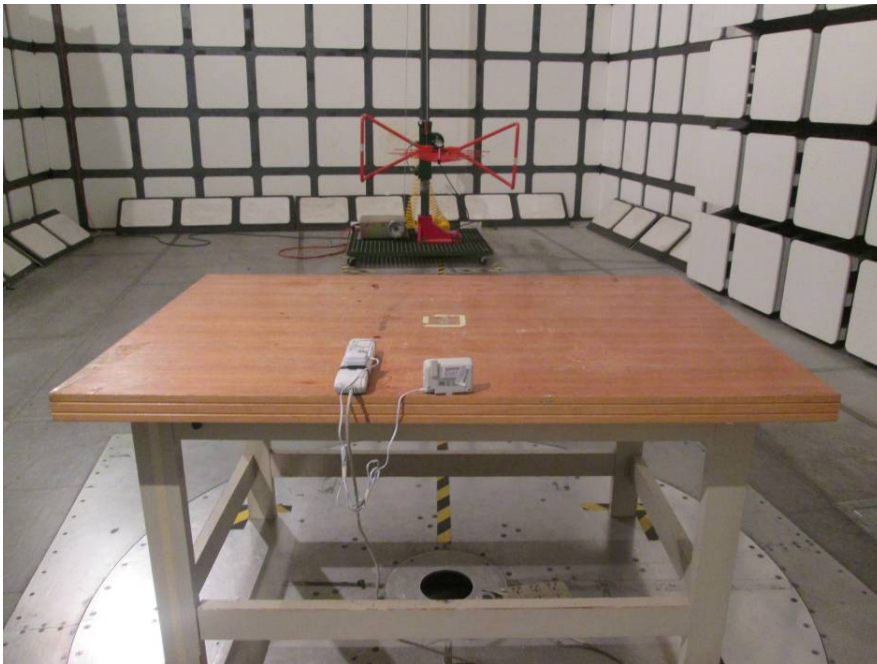
Radiated Emissions - Rear View (Below 1 GHz)
