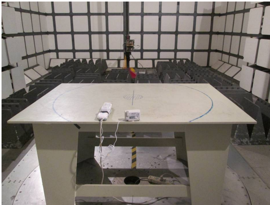
Radiated Emissions - Rear View (Above 1 GHz)
