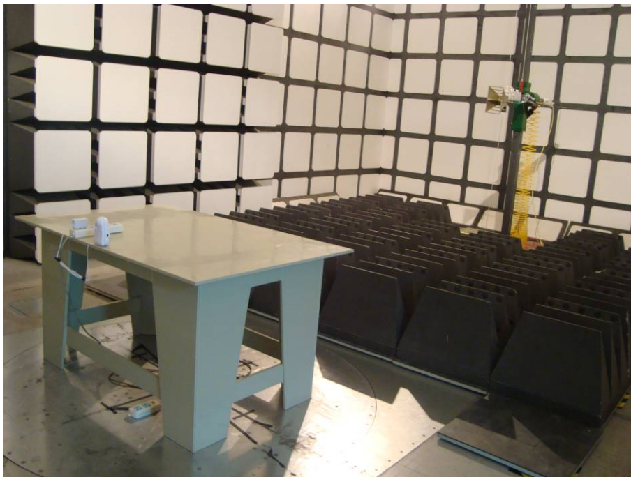
Above 1 GHz: Radiated Emissions - Rear View
