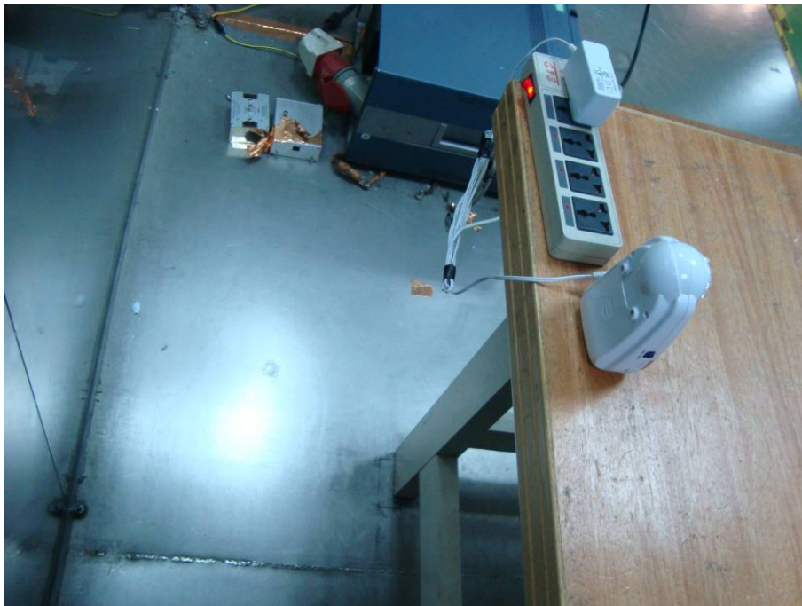
AC Line Conducted Emissions - Side View
