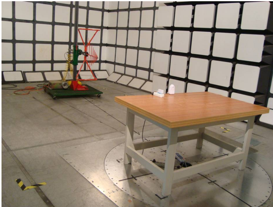
Below 1 GHz: Radiated Emissions - Front View
