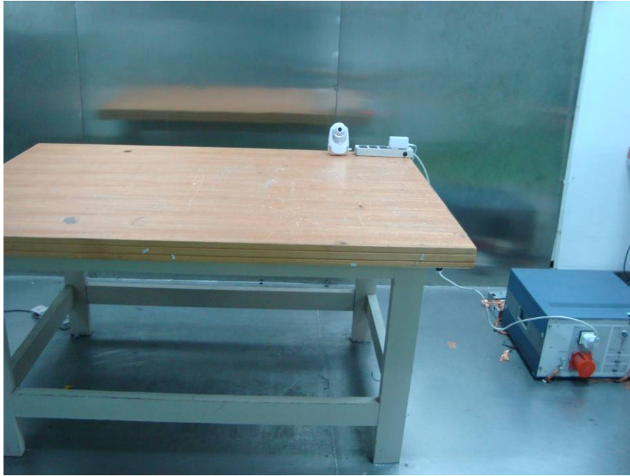
AC Line Conducted Emissions - Front View
