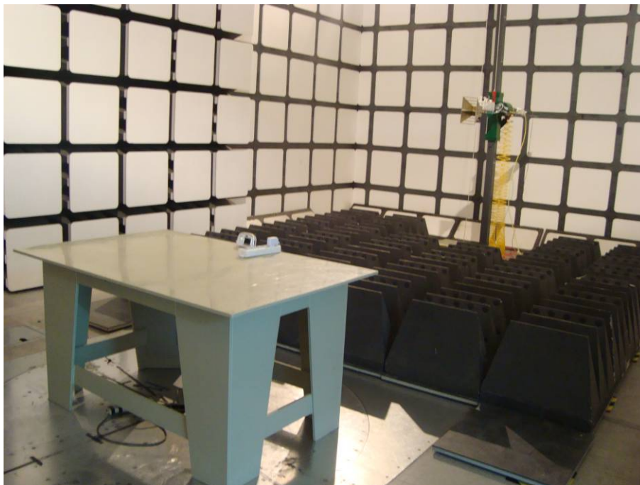
Above 1 GHz: Radiated Emissions - Rear View
