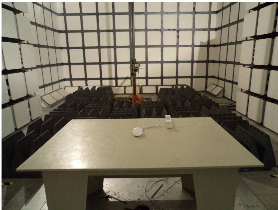
Radiated Emissions View (Above 1GHz)
