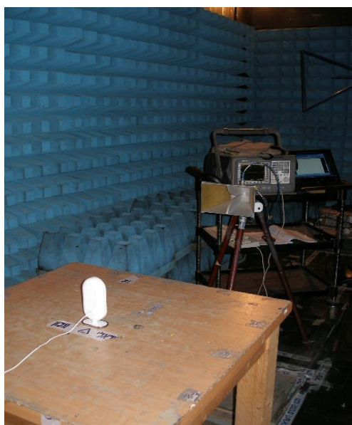
Photo 2. Spurious emissions test setup.
