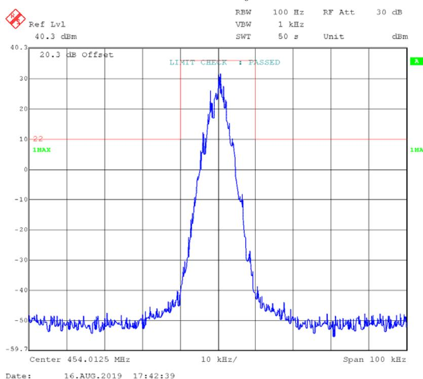
**4FSK,12.5 kHz, Low Power - Frequency 454.0125 MHz:****99% Occupied & 26 dB Bandwidth**
