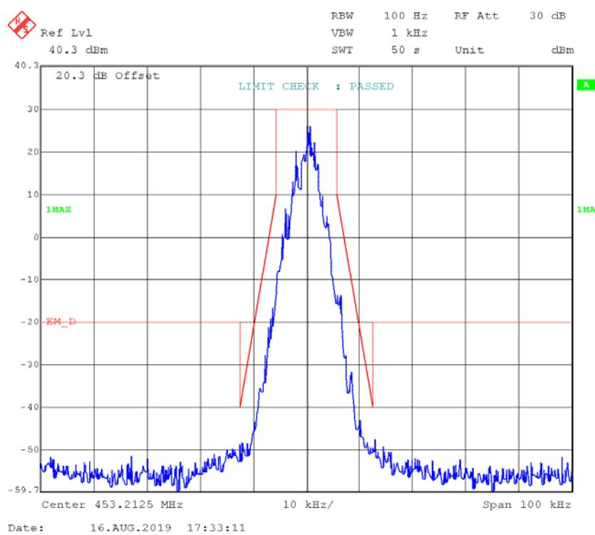
**Part 22****FM,12.5kHz, High Power - Frequency 454.0125 MHz:****99% Occupied& 26 dB Bandwidth**
