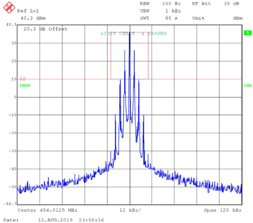
**FM,12.5kHz, Low Power – Frequency 454.0125 MHz:****99% Occupied & 26 dB Bandwidth**
