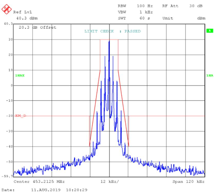
**4FSK,12.5kHz, High Power - Frequency 453.2125 MHz:****99% Occupied & 26 dB Bandwidth**
