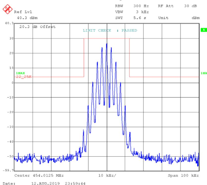
**4FSK,12.5 kHz, High Power - Frequency 454.0125 MHz:****99% Occupied & 26 dB Bandwidth**
