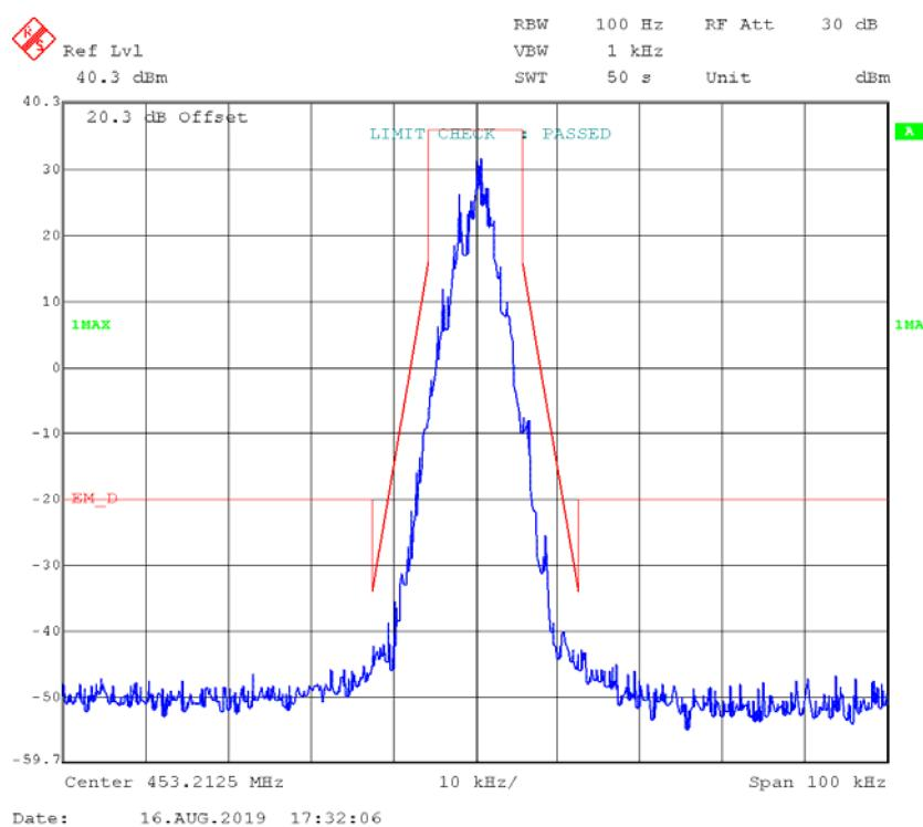
**4FSK,12.5kHz, Low Power - Frequency 453.2125 MHz:****99% Occupied & 26 dB Bandwidth**
