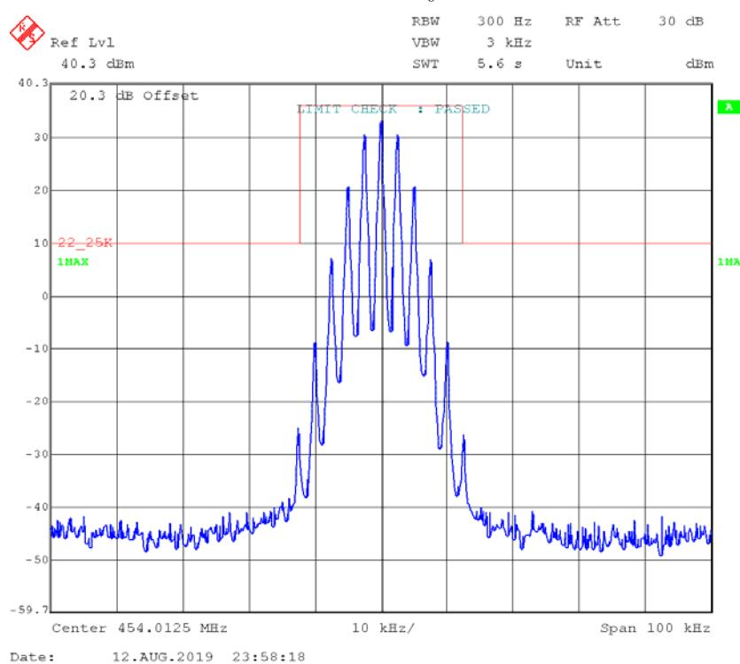
**FM, 25 kHz, Low Power – Frequency 454.0125 MHz:****99% Occupied & 26 dB Bandwidth**
