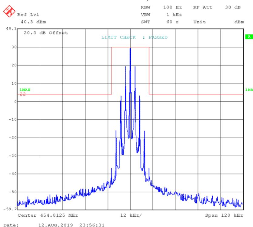
**FM,25kHz, High Power - Frequency 454.0125 MHz:****99% Occupied & 26 dB Bandwidth**
