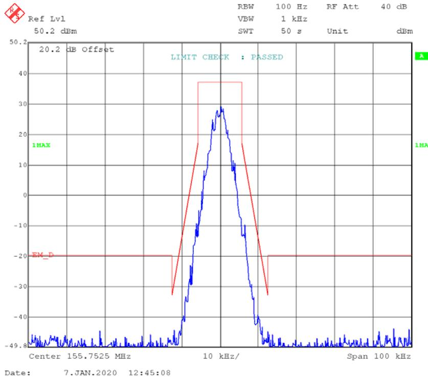
**4FSK,12.5kHz, Low Power - Frequency 155.7525 MHz:**
