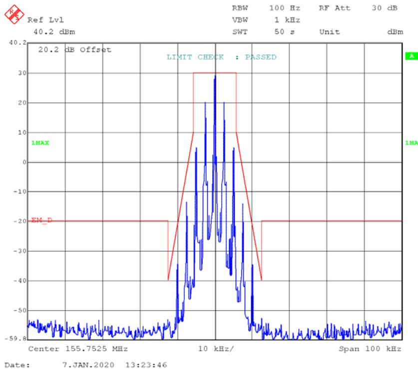
**4FSK,12.5kHz, High Power - Frequency 155.7525 MHz:**
