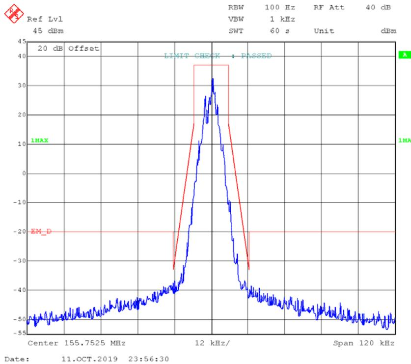
**4FSK,12.5kHz, Low Power - Frequency 155.7525 MHz:**
