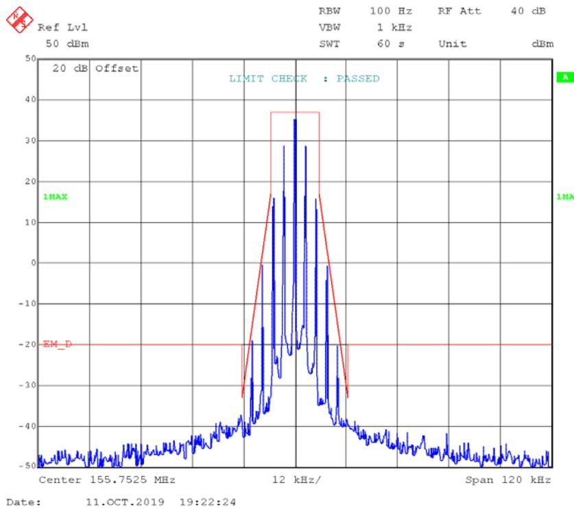
**4FSK,12.5kHz, High Power - Frequency 155.7525 MHz:**
