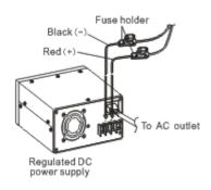
**2** Connect the transceiver's DC power connector to the connector on the DC power cable.
