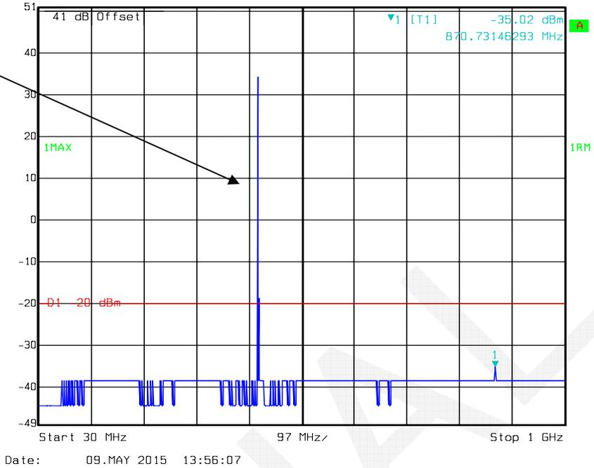
Marker 1 [T1] RBW 1 MHz RF Att 20 dB
