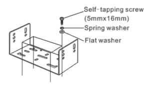
2 Position the transceiver, then insert and tighten the supplied hexagon SEMS screws (4) and flat washers (4).
