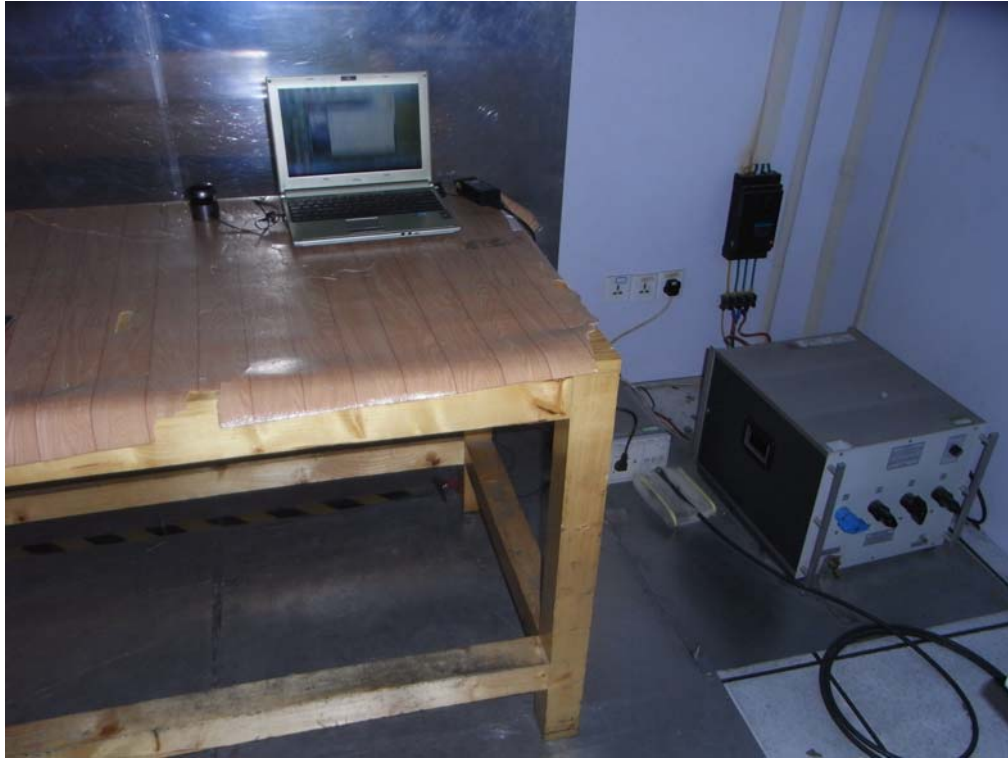
Test photo of Conducted emission ( Charging )
