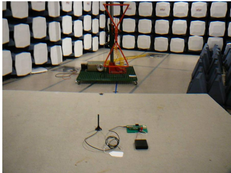
**13.3 Radiated Emission above 1 GHz – Front View**
