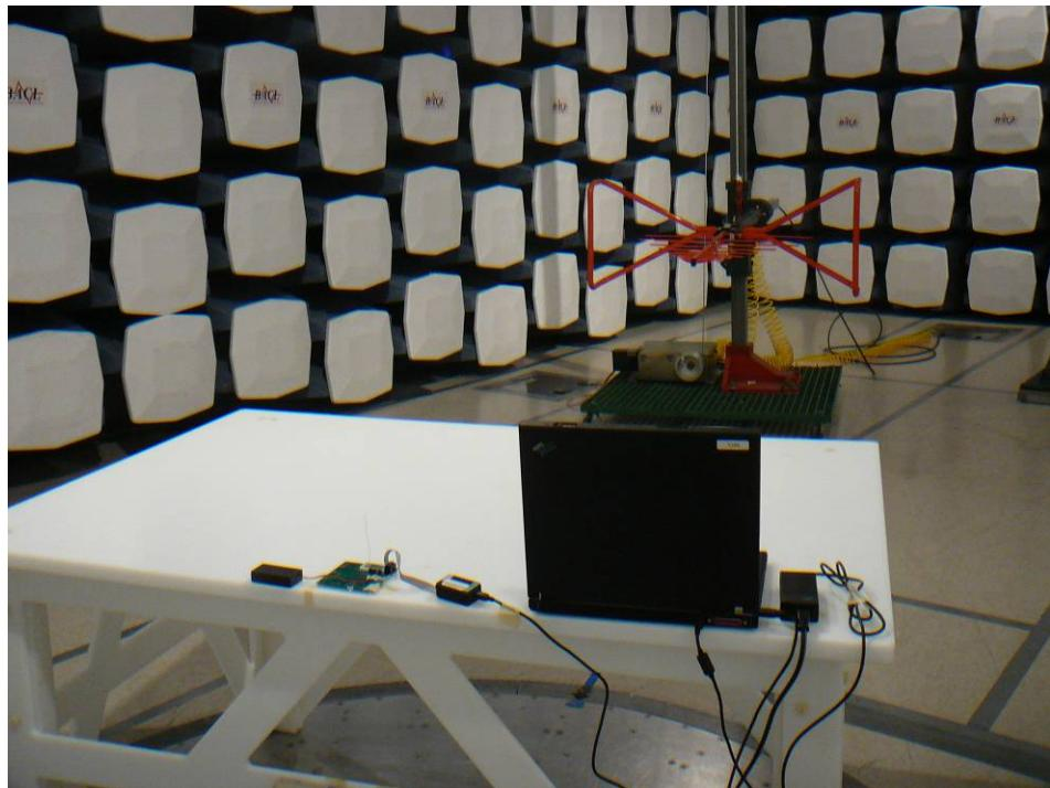
**15.5 TX Radiated Emission above 1 GHz Rear View at 3m**
