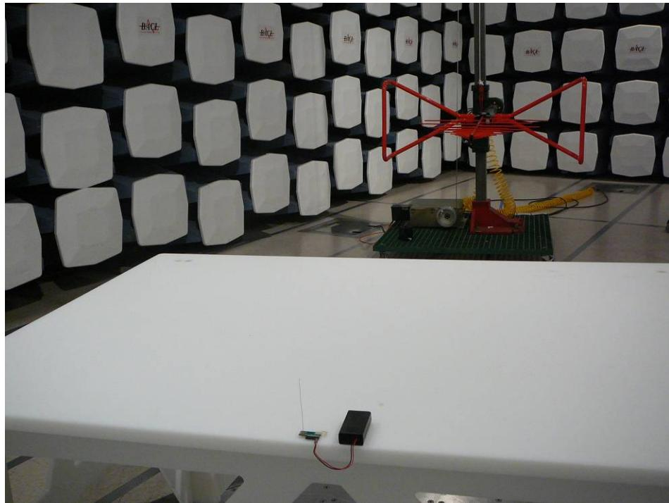
**15.8 RX Radiated Emission above 1 GHz Rear View at 3m**
