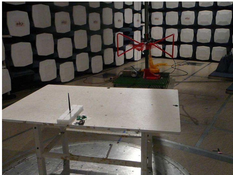
**14.6 Radiated Emission above 1 GHz Rear View (Dipole Antenna)**
