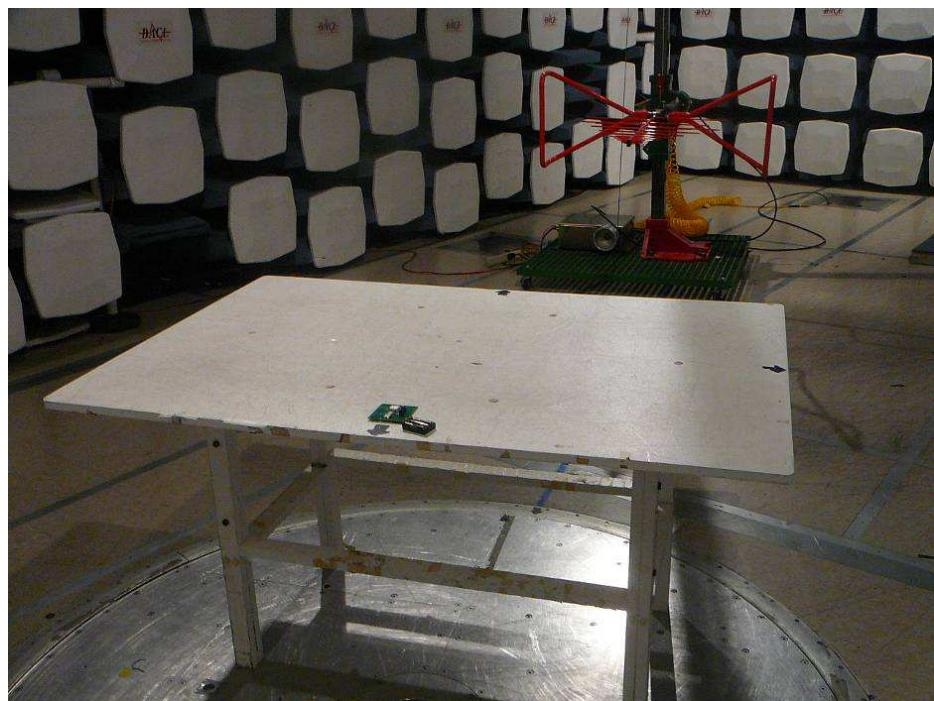
**14.3 Radiated Emission above 1 GHz Rear View (Wire Antenna)**
