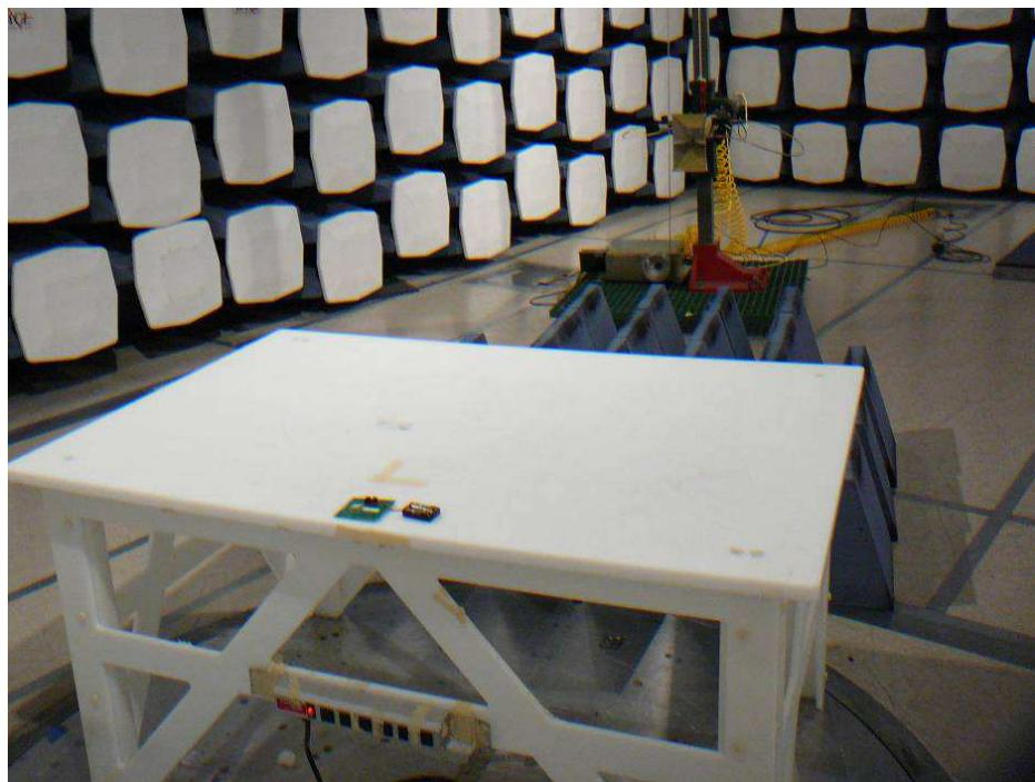
**14.4 Radiated Emission Front View (Dipole Antenna)**
