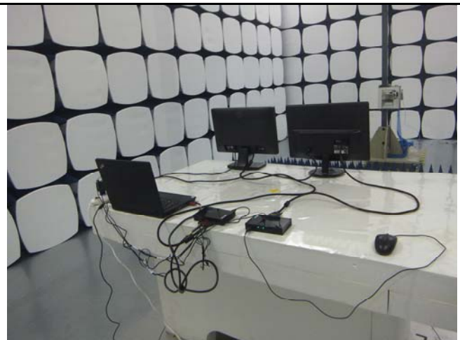
Radiated Spurious Emissions Test Setup Above 1GHz
