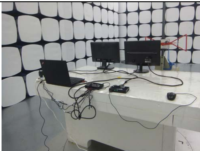
Radiated Spurious Emissions Test Setup Below 1GHz
