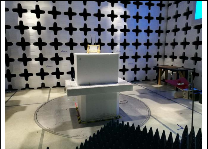
Radiated Emission Above 1G external antenna- Rear View
