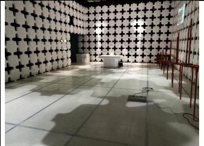
Radiated Emission Below 1G external antenna- Rear View
