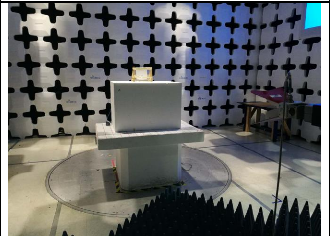
Radiated Emission Above 1G internal antenna- Rear View
