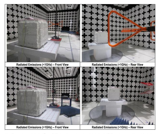
Note: The spurious emission in different EUT orientation was investigated, including the EUT standing up position and the laying down position. The EUT orientation shown in above setup photo is the worst-case position.
