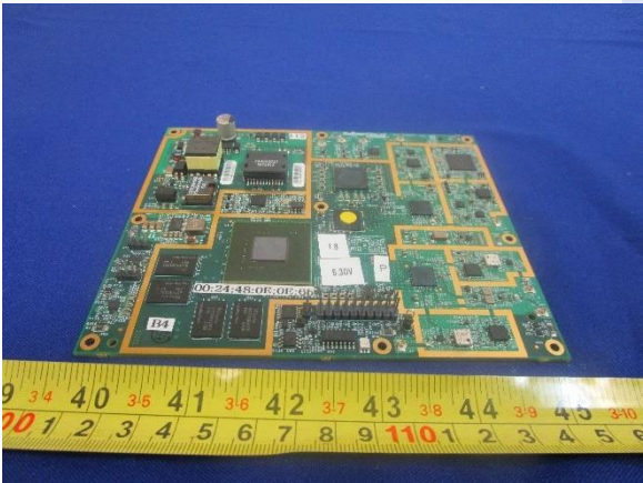
Picture 3: Main Board- Front View
