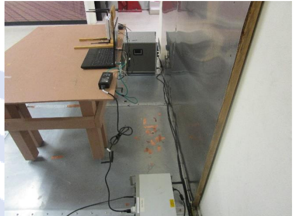
Picture 2: AC Conducted Emissions- Rear View
