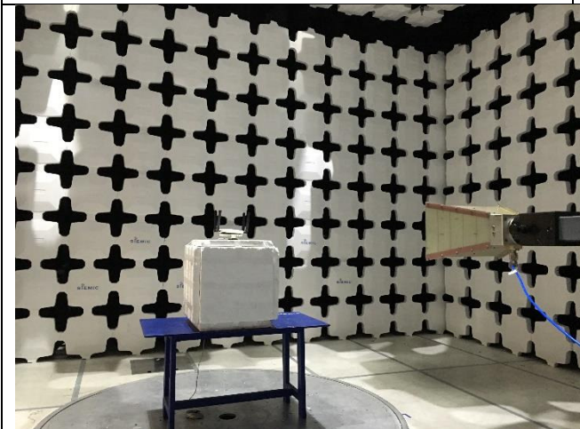
Radiated Emissions (>1GHz) – Front View
