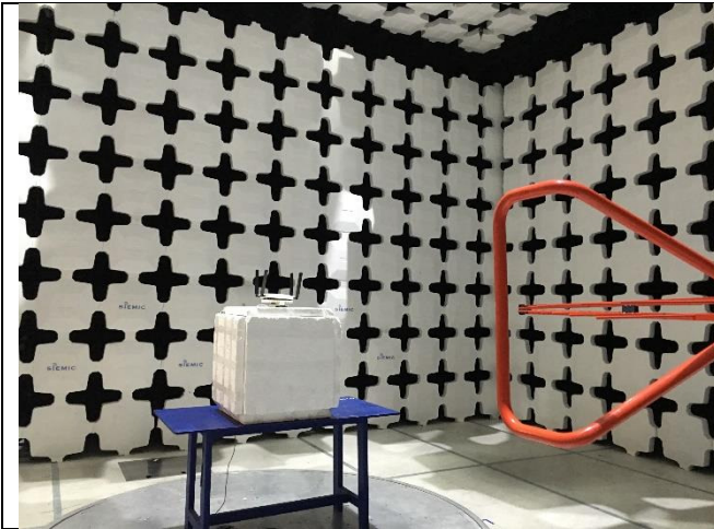
Radiated Emissions (<1GHz) – Front View
