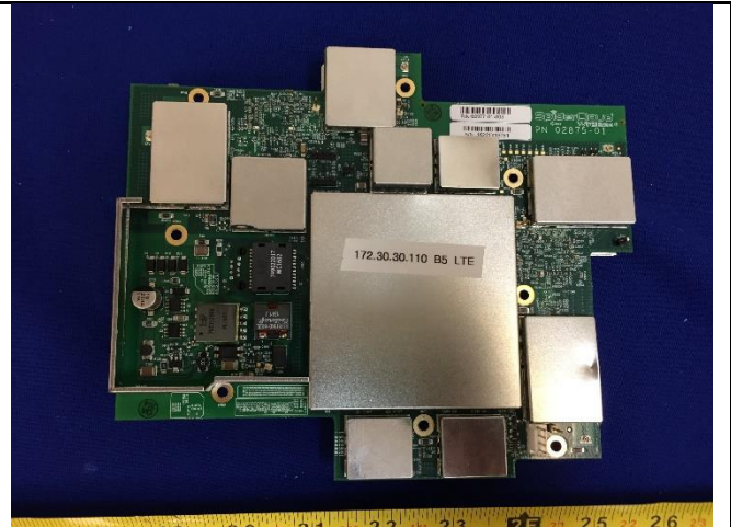
Main PCB with shielding - Top View
