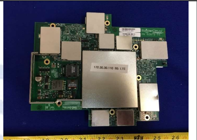
Main PCB with shielding - Top View
