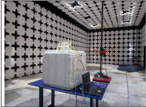
Radiated Emissions (<1GHz) – Front View
