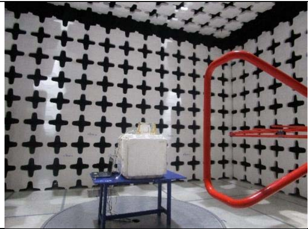
Radiated Emissions (<1GHz) – Rear View
