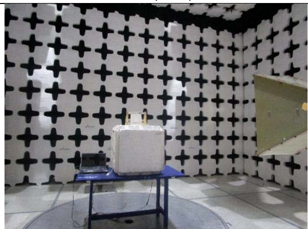
Radiated Emissions (>1GHz) – Rear View
