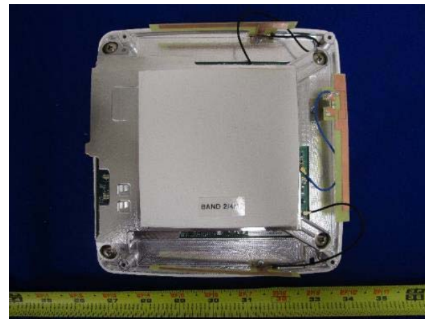
Internal Antenna View 1
