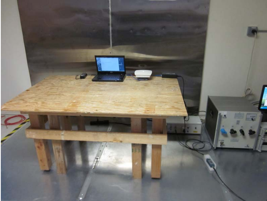
Conducted Emission Test Setup – Front View
