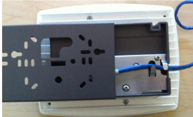
Figure 11 Slide the Mount Bracket onto the Pedestal Base
