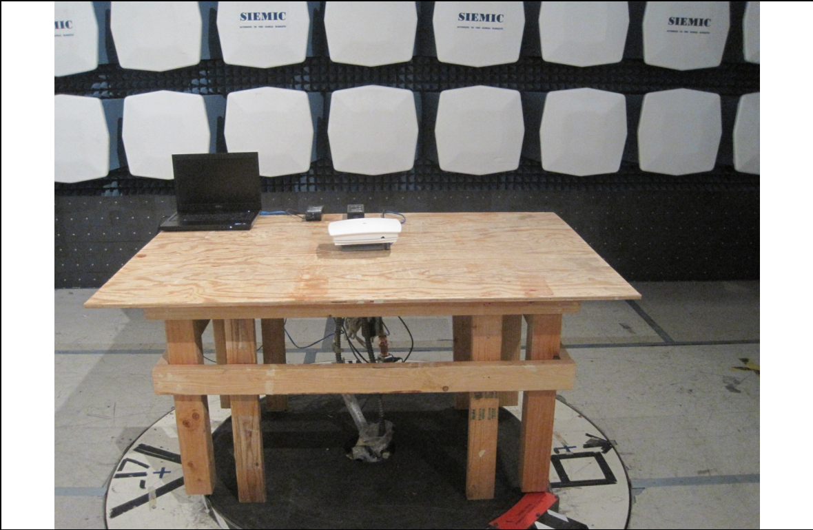
Radiated Emission Test Setup with patch antenna (Above 1GHz) - Front View (Internal Antenna)
