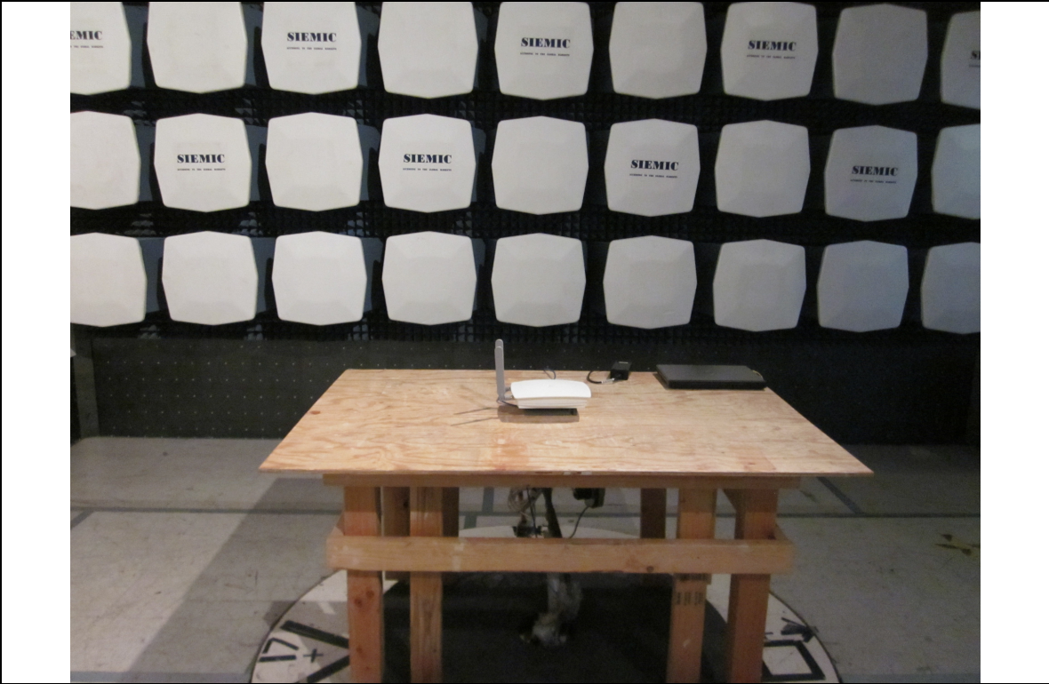
Radiated Emission Test Setup with patch antenna (Above 1GHz) - Front View (External Antenna)
