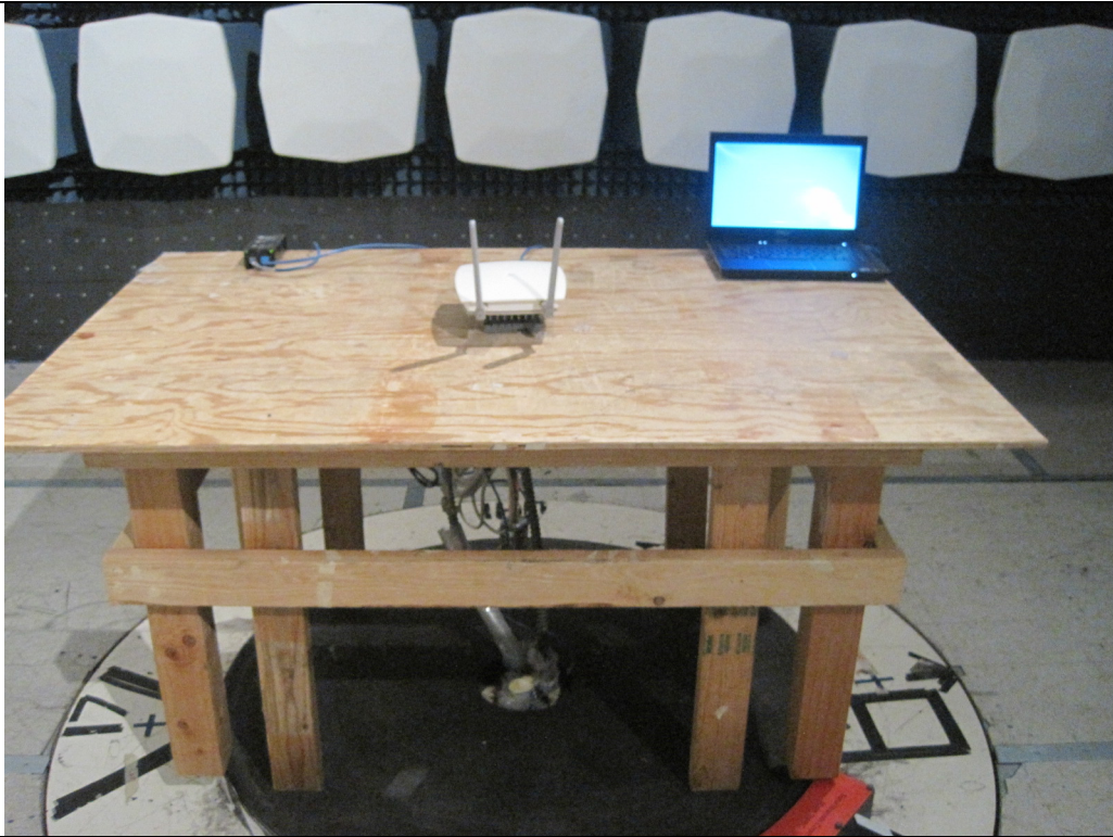
Radiated Emission Test Setup (30MHz – 1GHz) - Front View (External Antenna)
