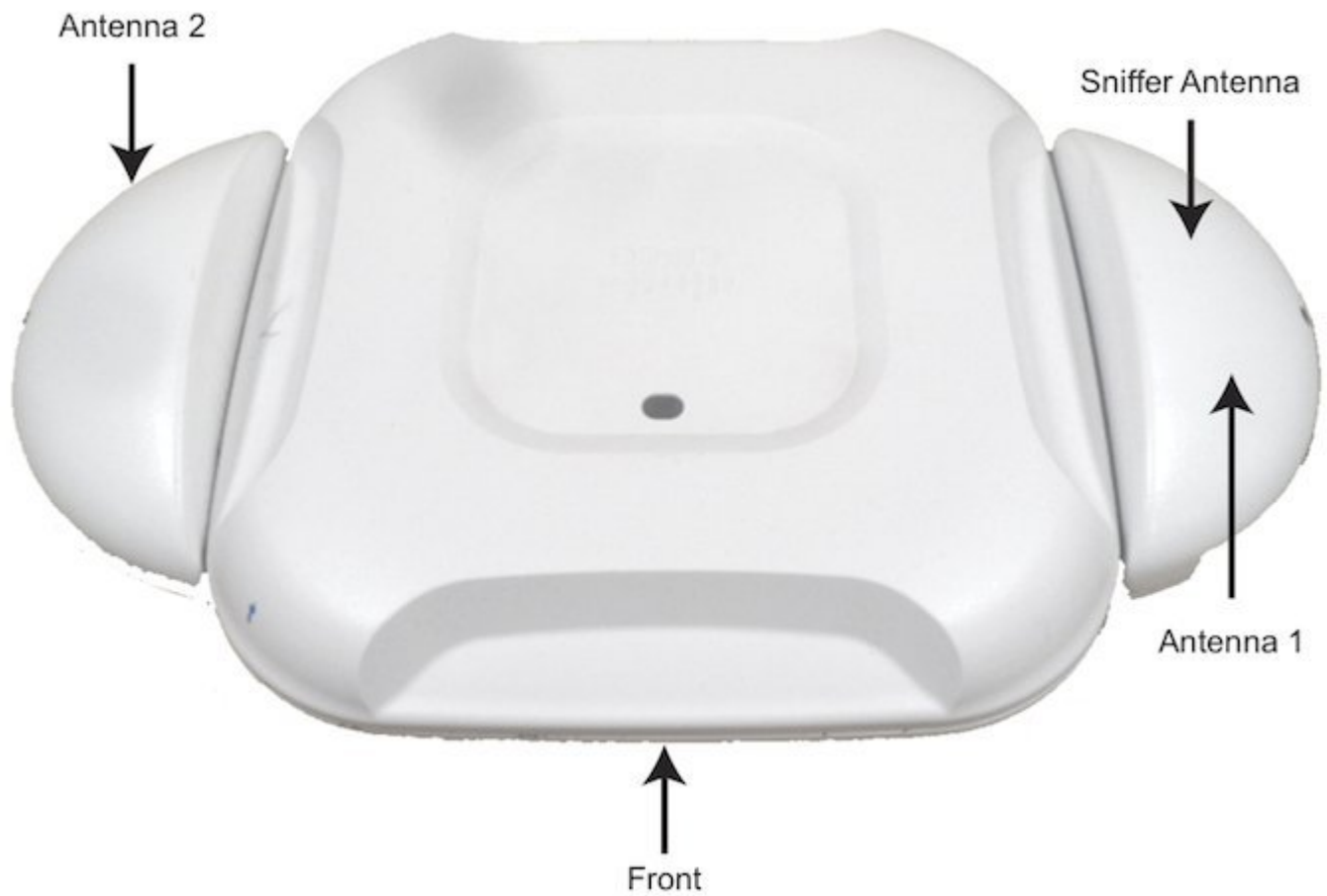
Figure 6: Orientation and Antenna Locations
