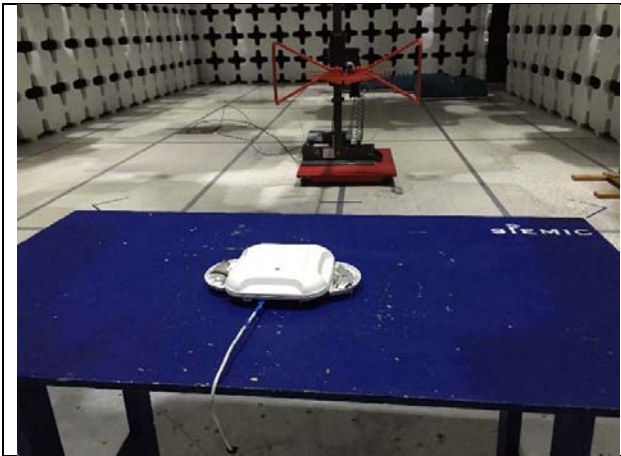
Radiated Emissions (<1GHz) – Front View
