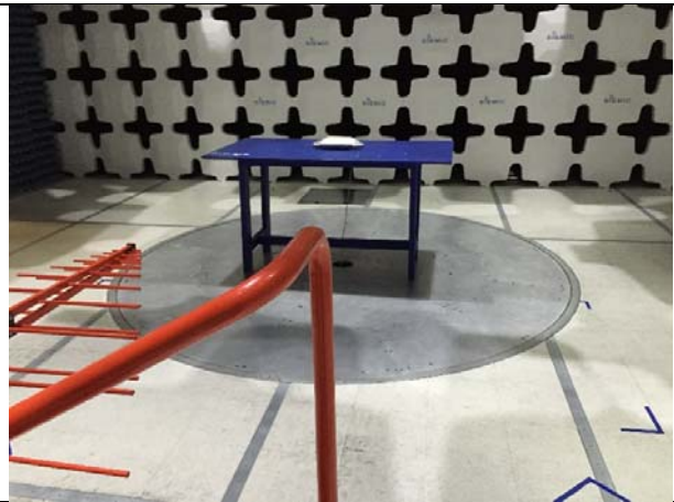
Radiated Emissions (<1GHz) – Rear View
