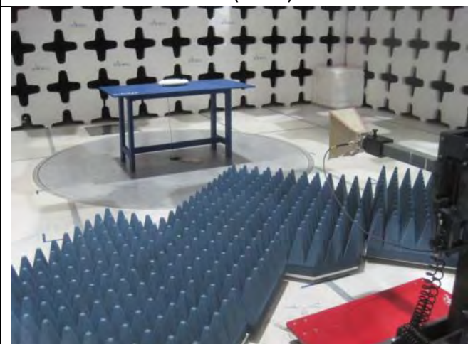
Radiated Emissions (>1GHz) – Front View
