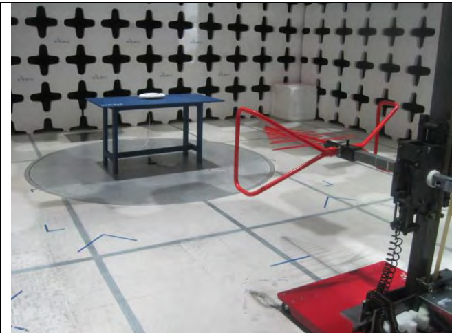
Radiated Emissions (<1GHz) – Front View
