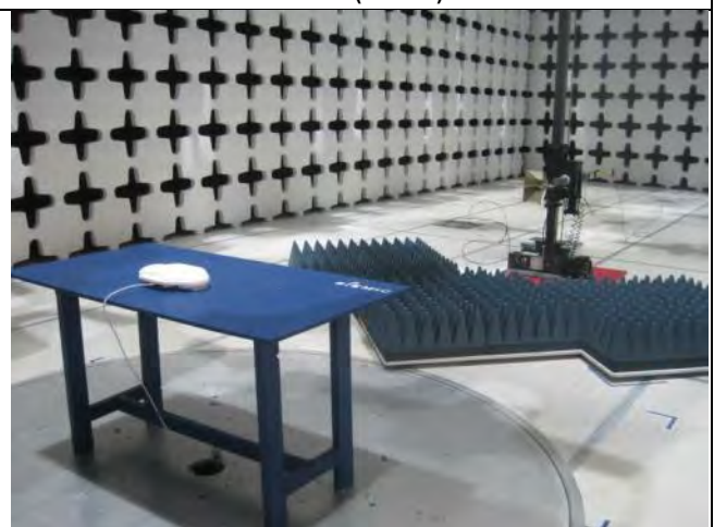
Radiated Emissions (>1GHz) – Rear View
