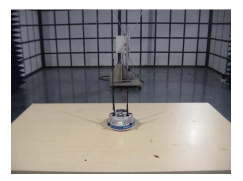
Radiation Emission Test Setup (Above 1GHz)
