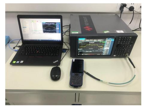
1.3 Set-up for Spurious Emissions below 1GHz
