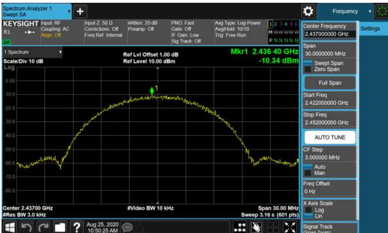
Figure 14: Power Spectral Density, 802.11b, 2437MHz
