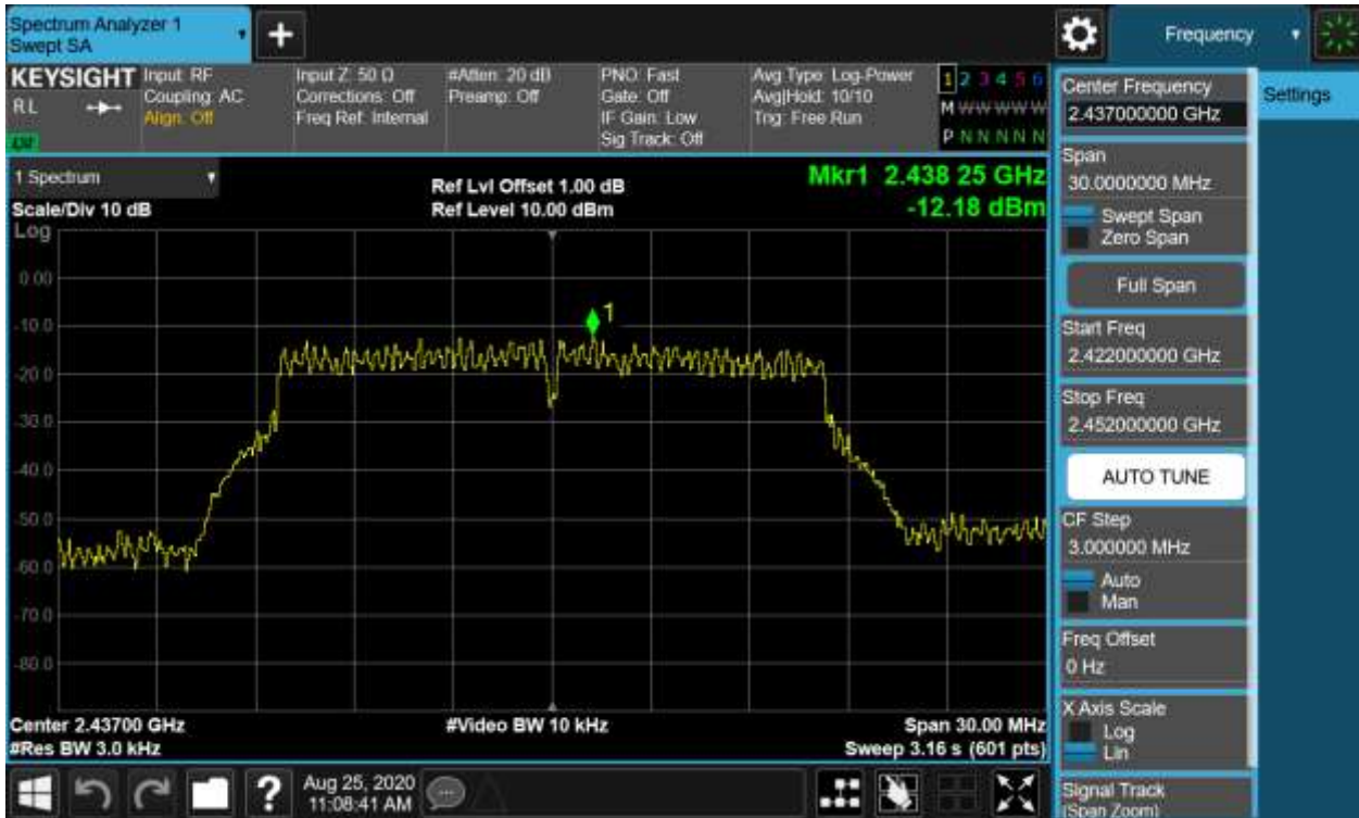
Figure 17: Power Spectral Density, 802.11g, 2437MHz
