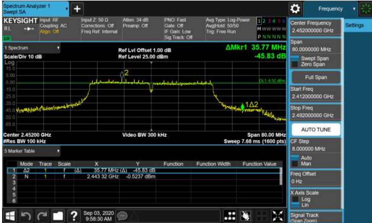
Figure 12: 6dB Bandwidth and 99% Bandwidth, 802.11n(HT40), 2452MHz
