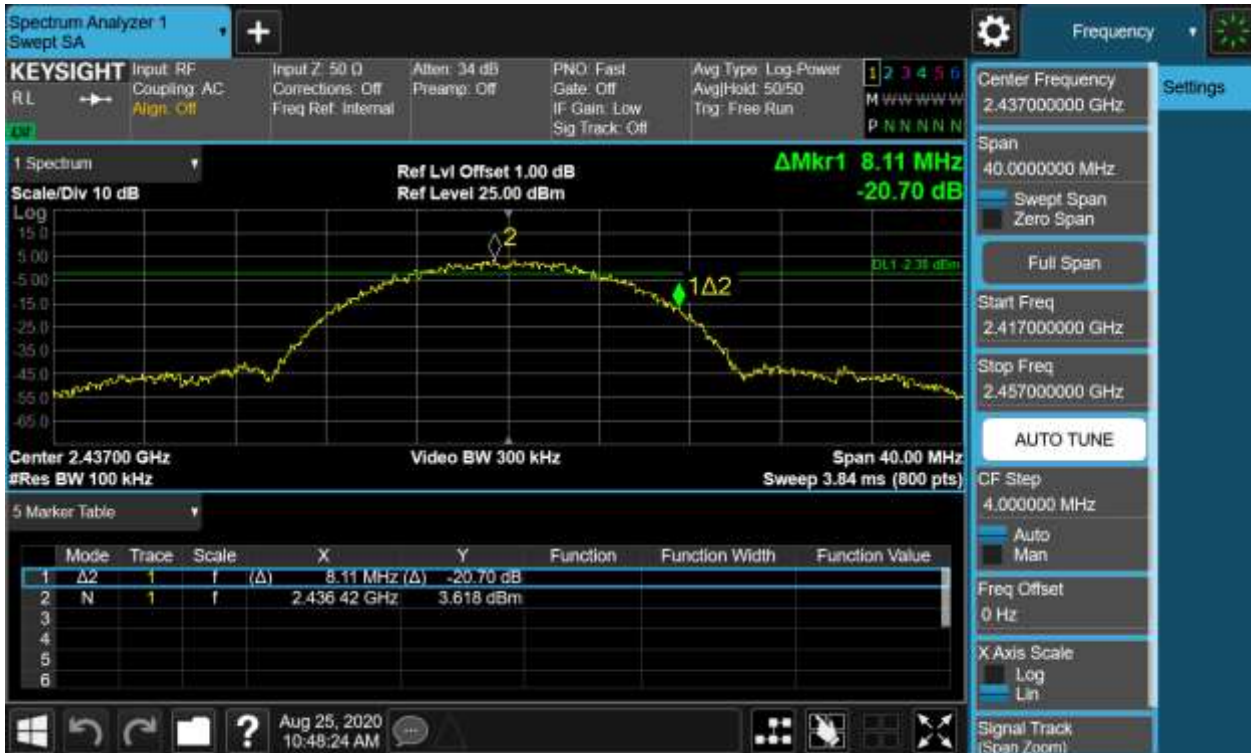
Figure 2: 6dB Bandwidth and 99% Bandwidth, 802.11b, 2437MHz
