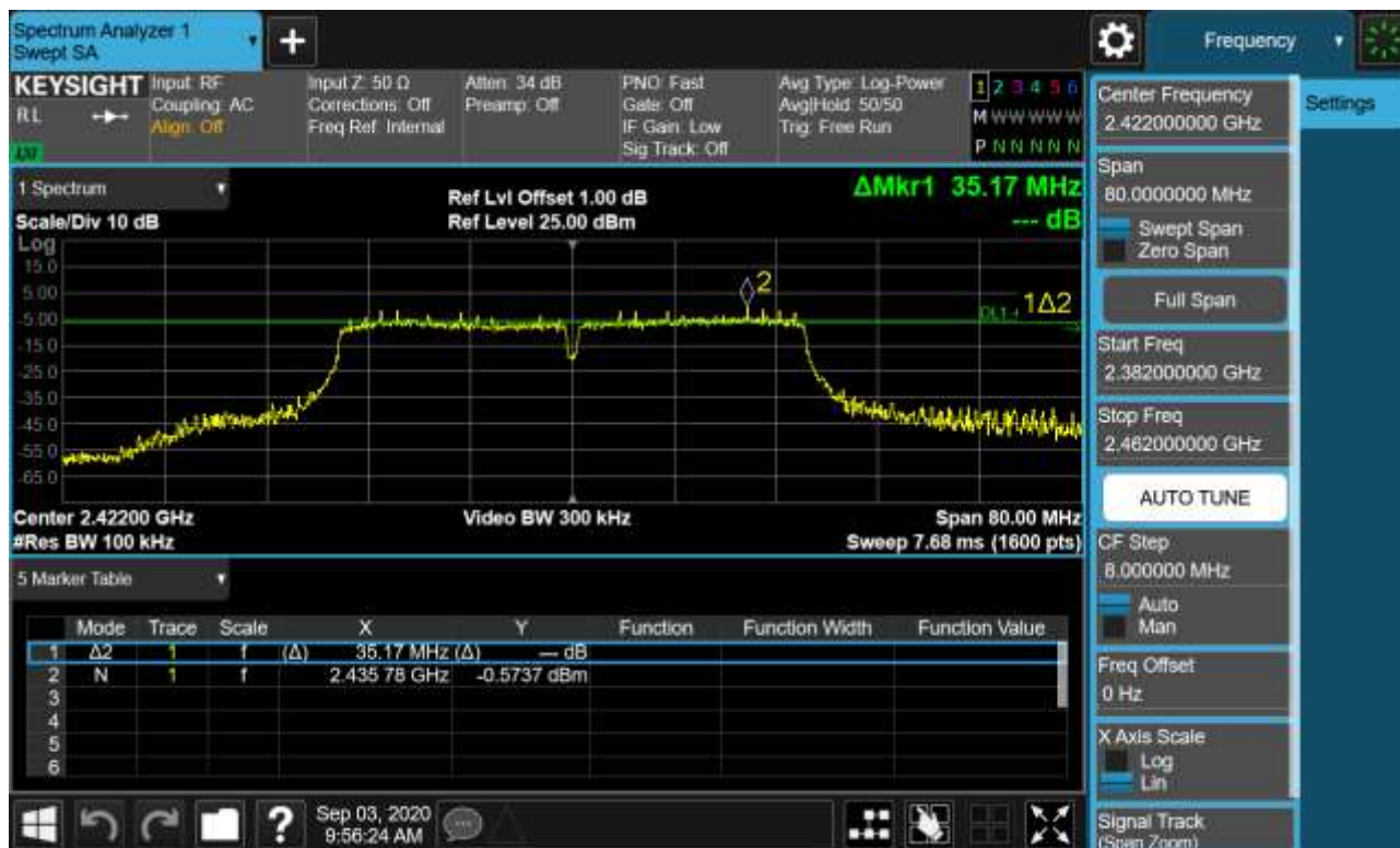
Figure 10: 6dB Bandwidth and 99% Bandwidth, 802.11n(HT40), 2422MHz
