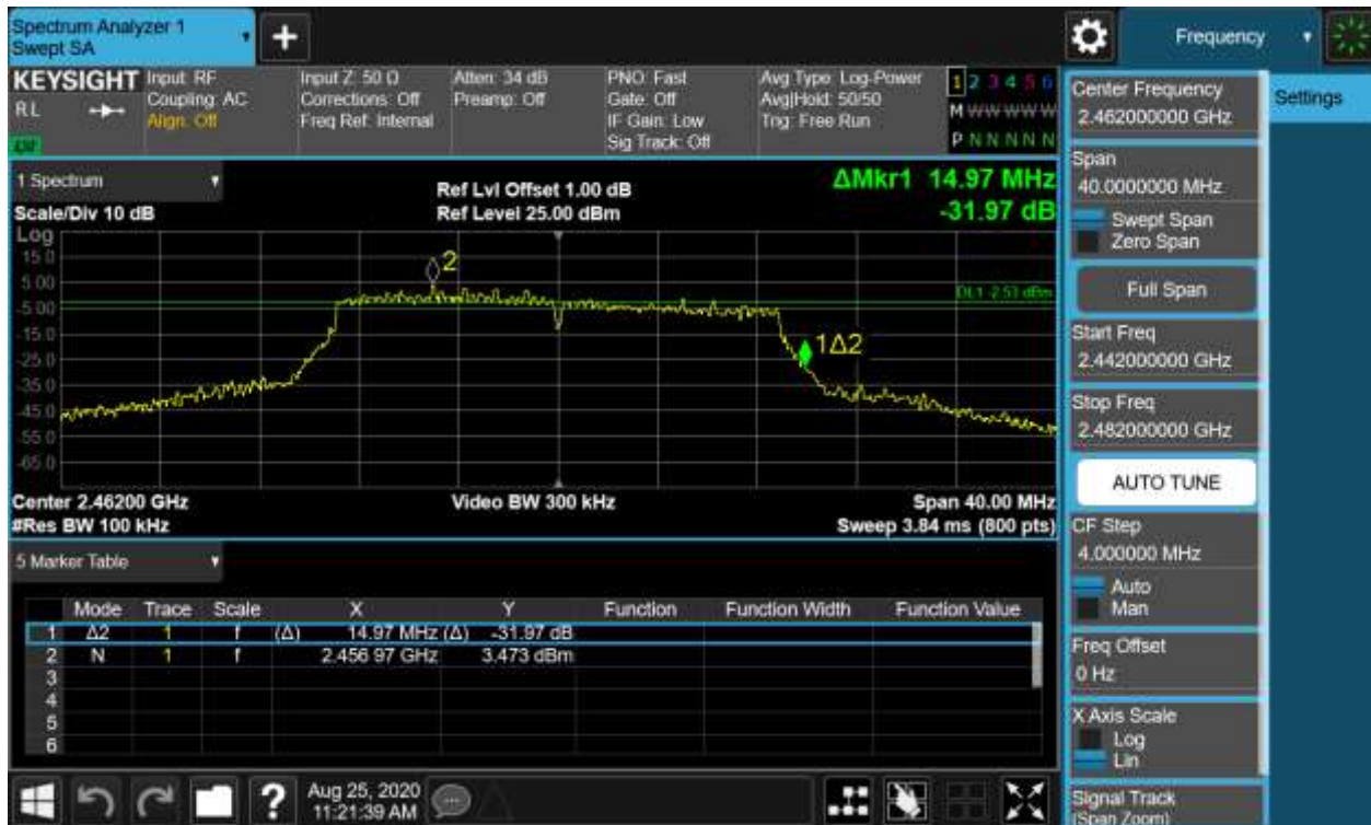
Figure 9: 6dB Bandwidth and 99% Bandwidth, 802.11n(HT20), 2462MHz
