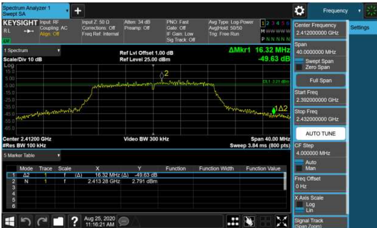
Figure 7: 6dB Bandwidth and 99% Bandwidth, 802.11n(HT20), 2412MHz
