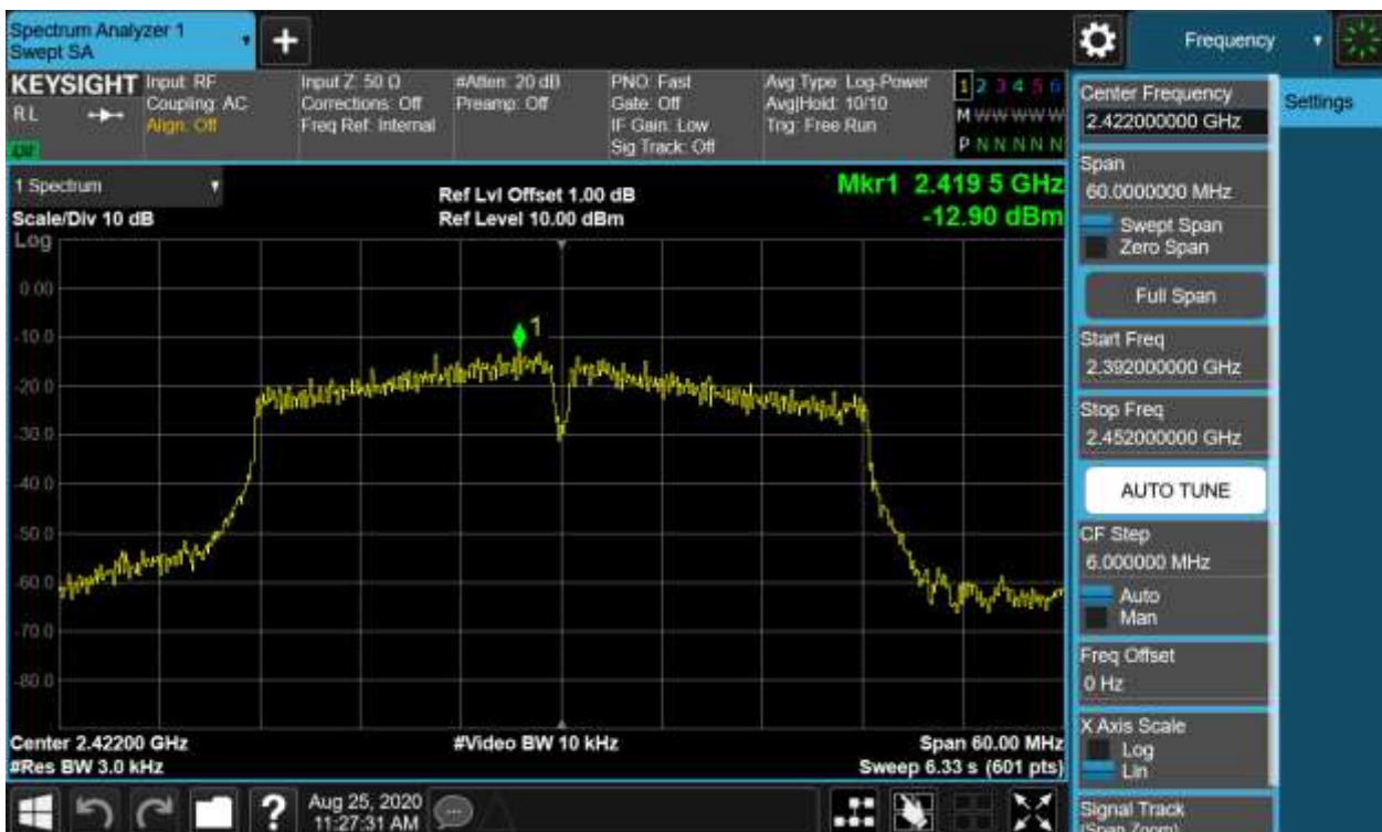
Figure 22: Power Spectral Density, 802.11n(HT40), 2422MHz
