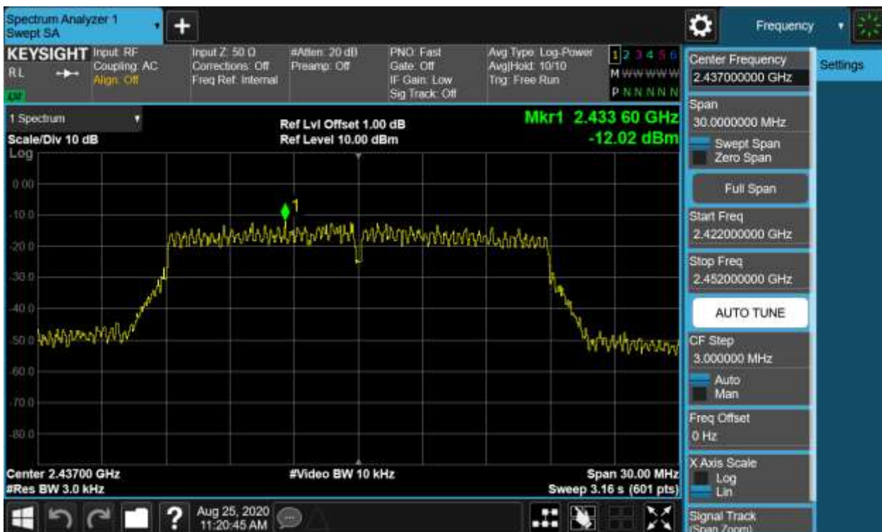
Figure 20: Power Spectral Density, 802.11n(HT20), 2437MHz
