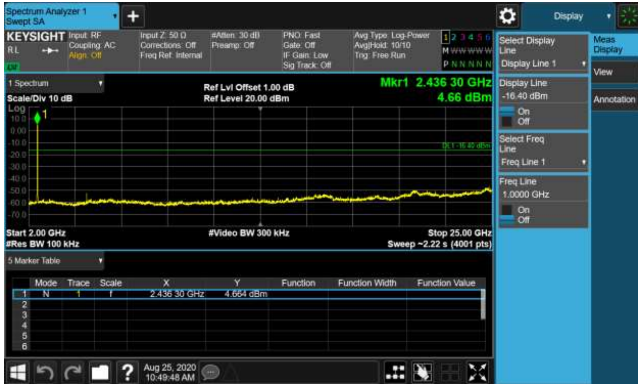
Figure 27: Conducted Spurious Emission & Authorized-band band-edge, 802.11b, 2462MHz Carrier Level
