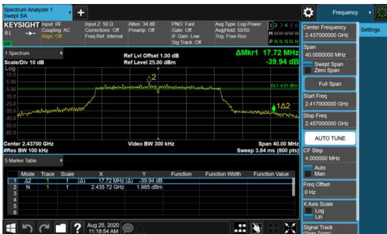
Figure 8: 6dB Bandwidth and 99% Bandwidth, 802.11n(HT20), 2437MHz
