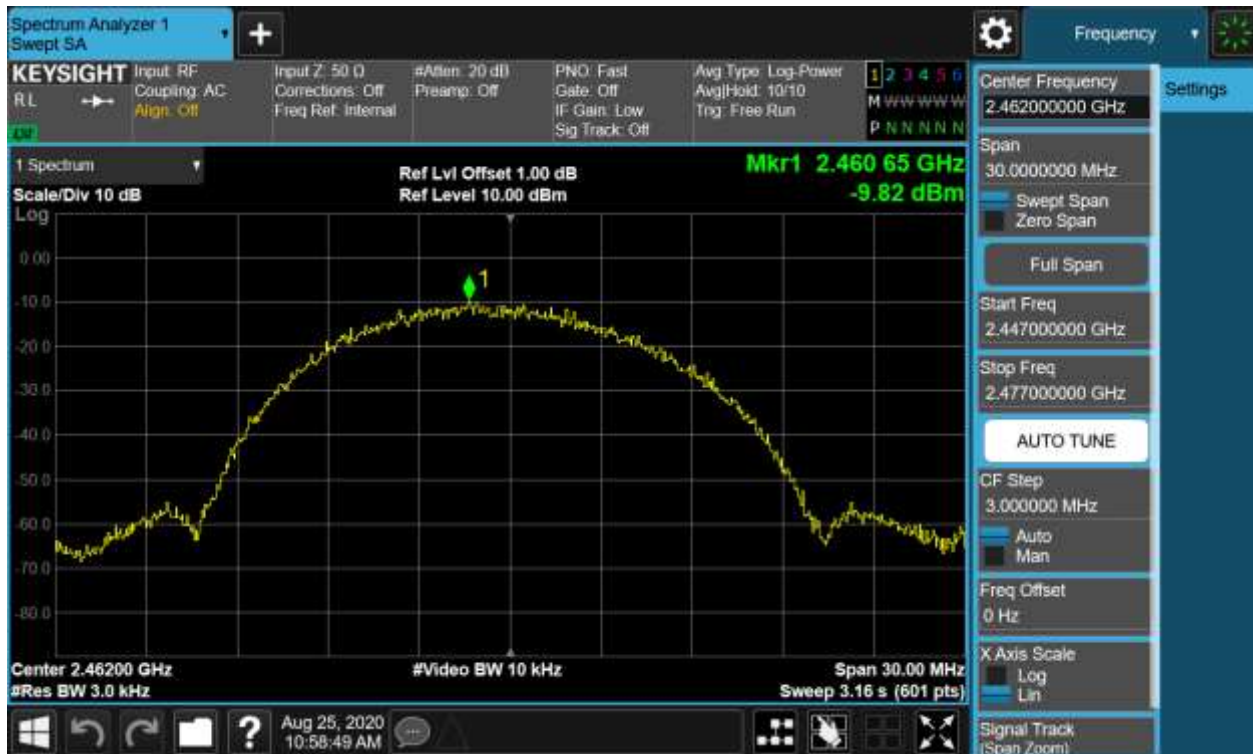
Figure 15: Power Spectral Density, 802.11b, 2462MHz
