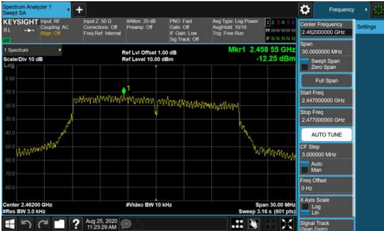
Figure 21: Power Spectral Density, 802.11n(HT20), 2462MHz
