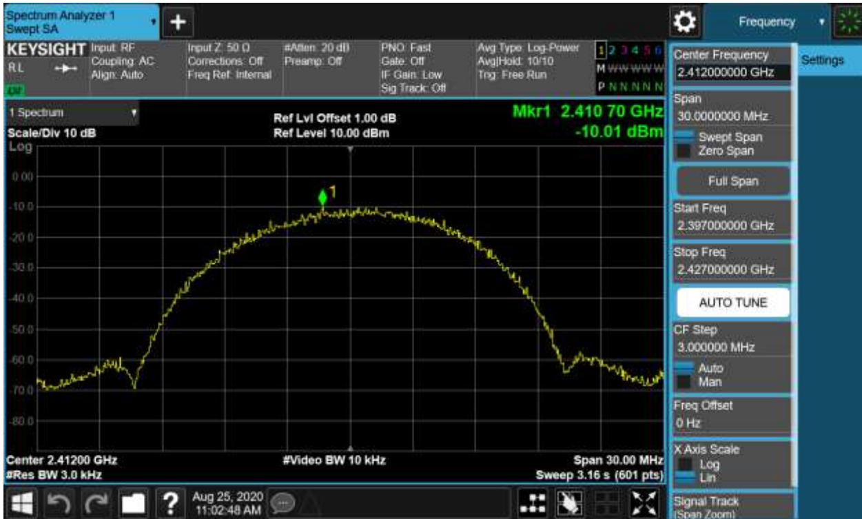
Figure 13: Power Spectral Density, 802.11b, 2412MHz
