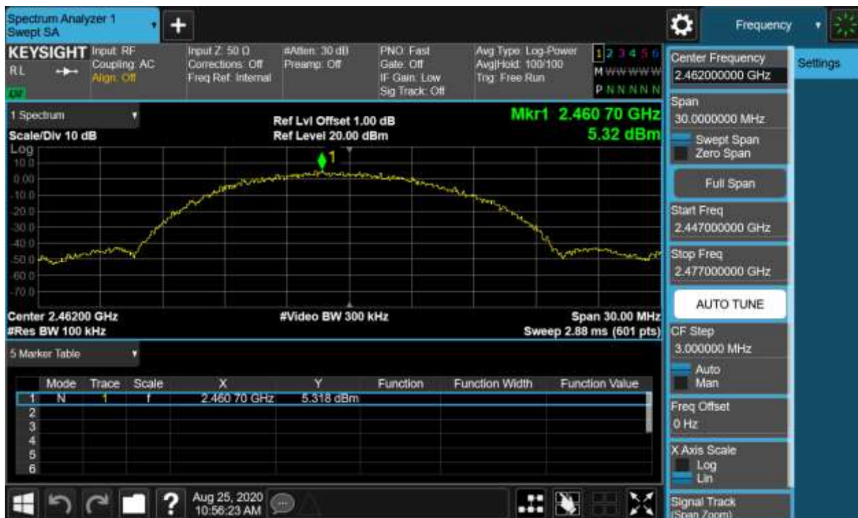
Figure 27: Conducted Spurious Emission & Authorized-band band-edge, 802.11b, 2462MHz Carrier Level
