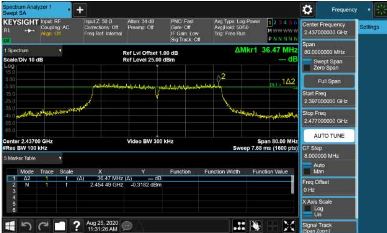
Figure 11: 6dB Bandwidth and 99% Bandwidth, 802.11n(HT40), 2437MHz
