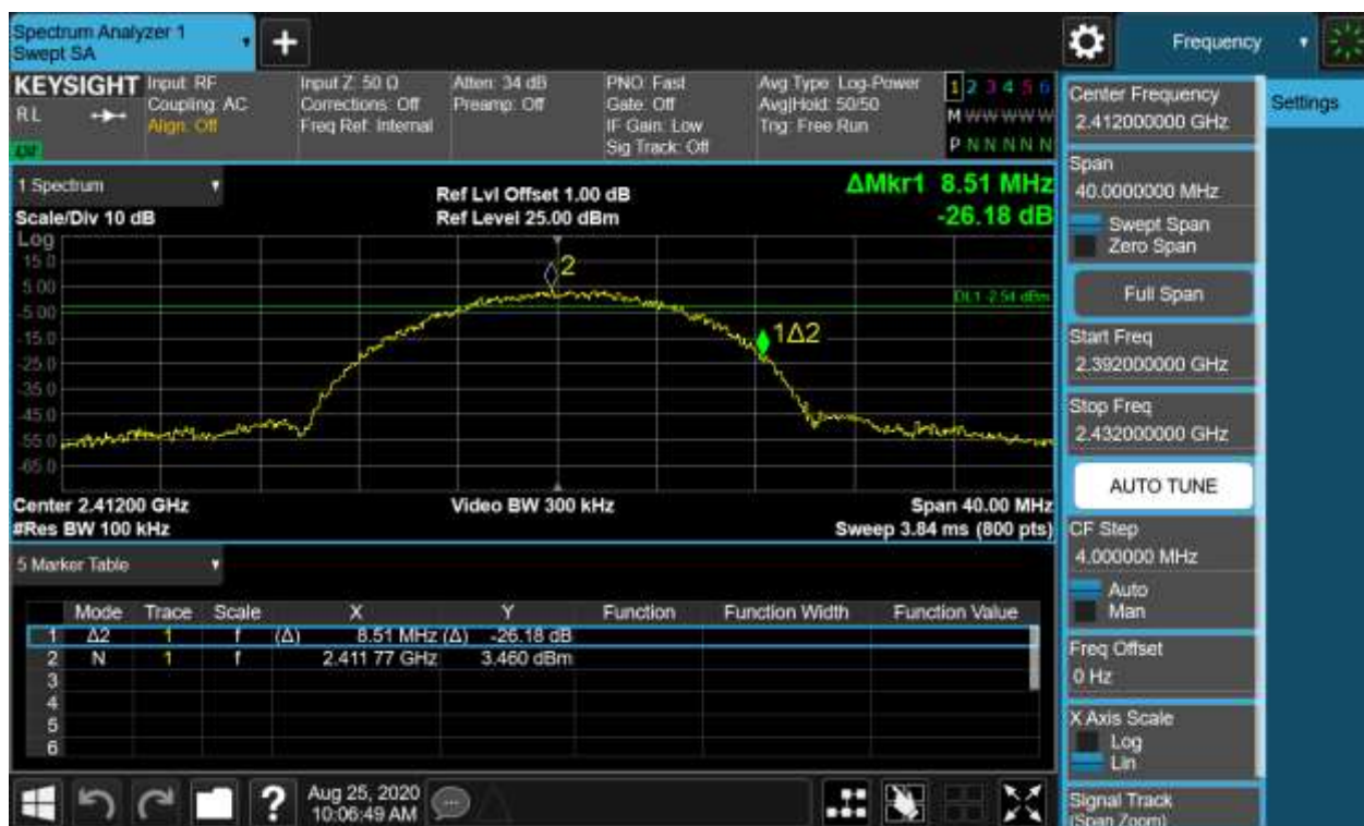
Figure 1: 6dB Bandwidth and 99% Bandwidth, 802.11b, 2412MHz
