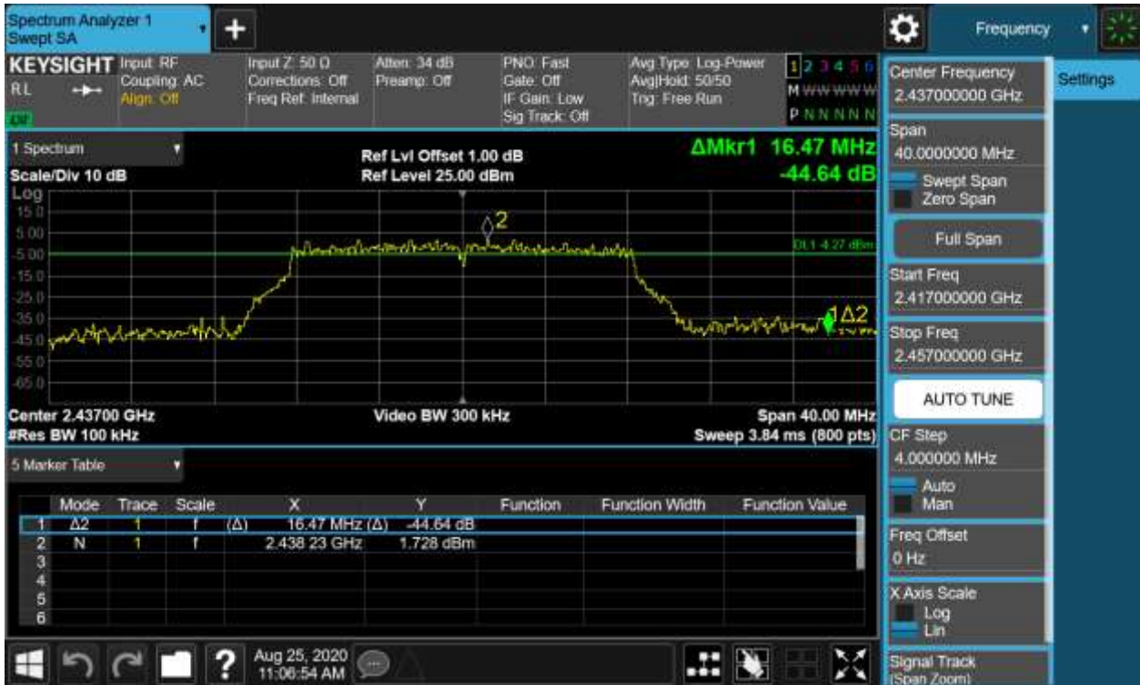
Figure 5: 6dB Bandwidth and 99% Bandwidth, 802.11g, 2437MHz
