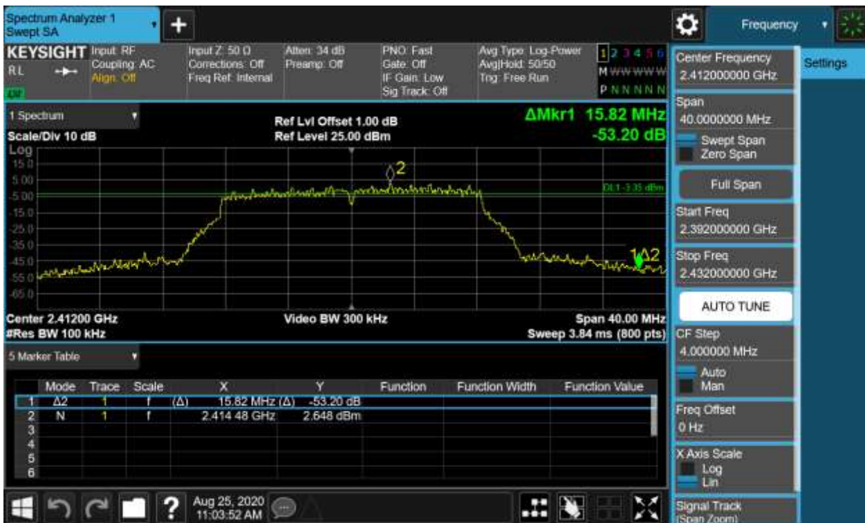
Figure 4: 6dB Bandwidth and 99% Bandwidth, 802.11g, 2412MHz
