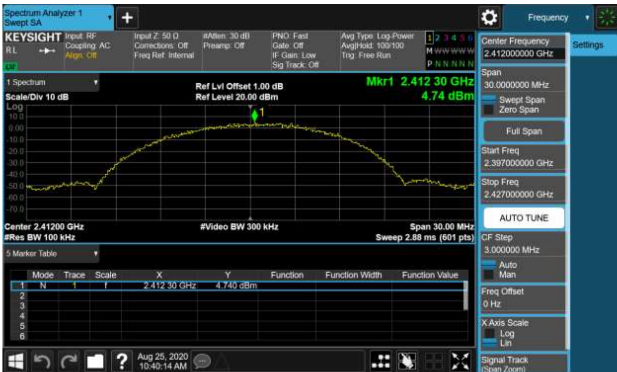
Figure 25: Conducted Spurious Emission & Authorized-band band-edge, 802.11b, 2412MHz Carrier Level
