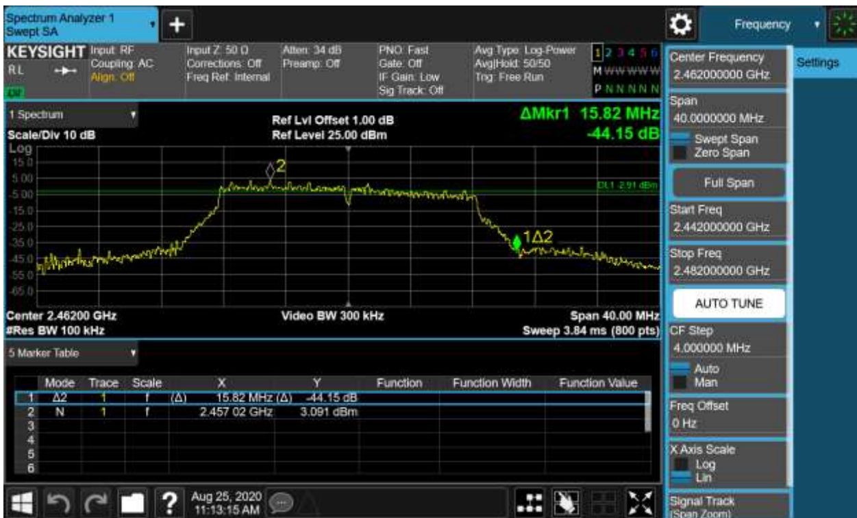
Figure 6: 6dB Bandwidth and 99% Bandwidth, 802.11g, 2462MHz
