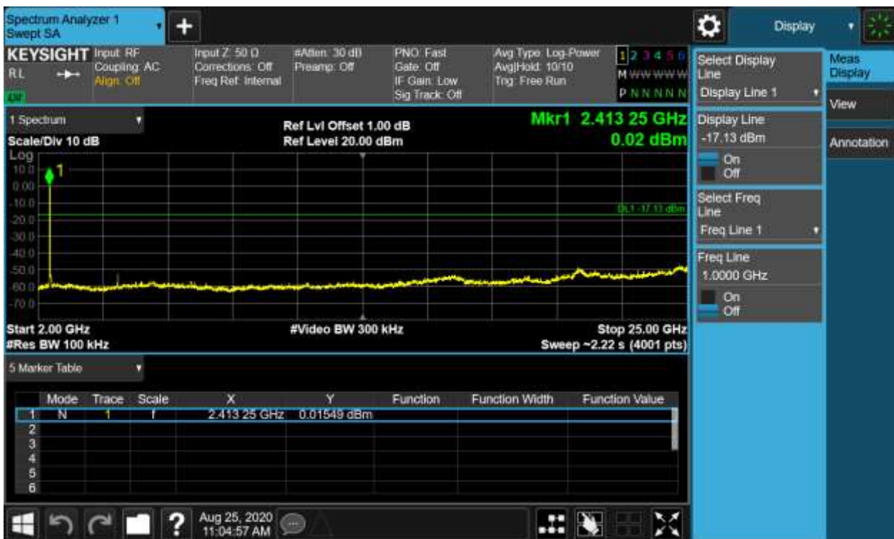
Figure 29: Conducted Spurious Emission & Authorized-band band-edge, 802.11g, 2437MHz
