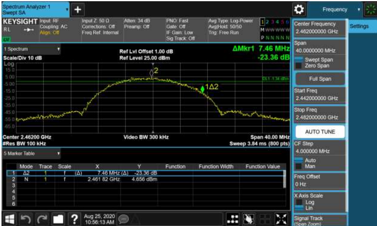
Figure 3: 6dB Bandwidth and 99% Bandwidth, 802.11b, 2462MHz
