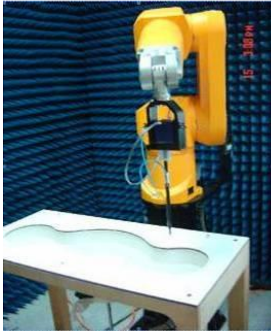
Photo 1: SAR measurement System
