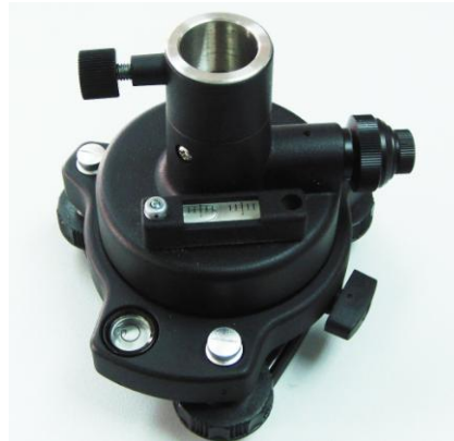
Fig. 3.15 – Tribrach and adapter with optical plummer
