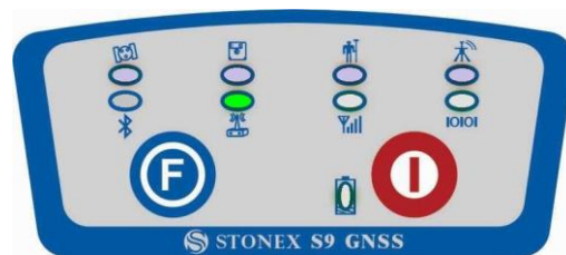
Fig 2.16 - S9III internal radio led
